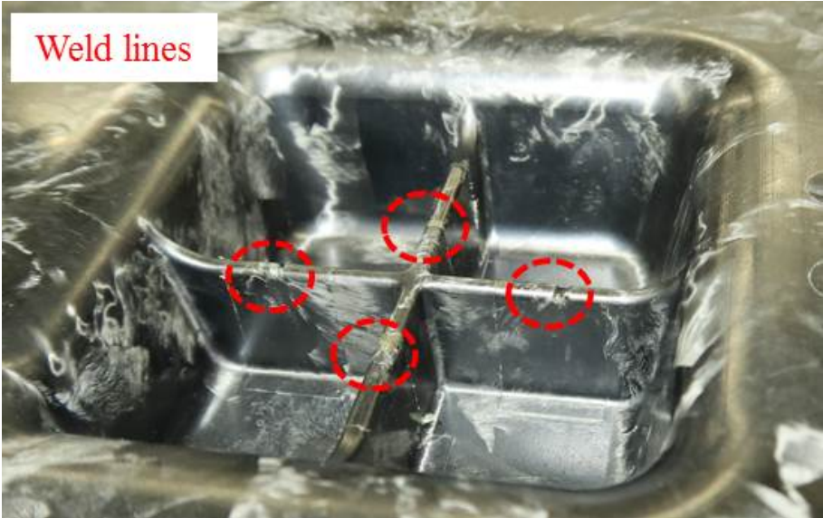
Figure 11. Formulation of weld lines in test
