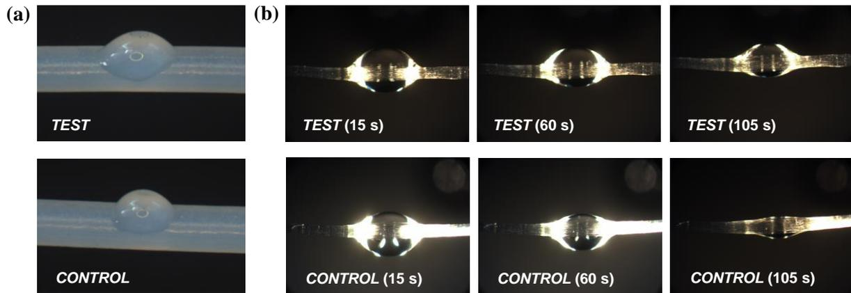
**Figure 4.** (a) Nylon 6,6 filament (1.6 mm diameter), with water droplets: the test sample was previously subjected to 54 MPa, 20 h creep and, compared with the (unstressed) control, shows lower contact angle, indicating reduced hydrophobicity; (b) nylon 6,6 yarn (140 filaments, 27 μm diameter), with water droplets: the test sample was previously subjected to 330 MPa, 24 h creep and, compared with the (unstressed) control, shows slower wicking, suggesting reduced hydrophobicity.
