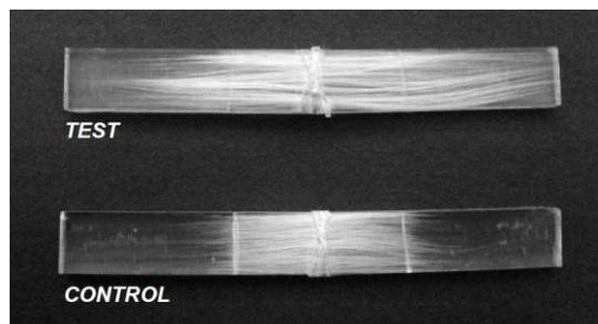
**Figure 3.** Typical appearance of test (VPPMC) and control (unstressed) samples following impact testing; note the greater region of fibre-matrix debonding in the test sample [9].
