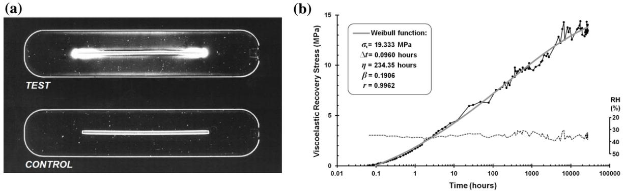
**Figure 2.** (a) nylon 6,6 monofilaments (1.6 mm diameter) moulded in polyester resin samples (150 × 80 × 2 mm) under cross-polarised light: a stress pattern can be clearly seen in the ‘test’ sample due to viscoelastic recovery (from 60 MPa 24 h creep), in contrast with the (unstressed) ‘control’ sample [13]; (b) viscoelastic recovery stress output (force exerted across fibres) from nylon 6,6 yarn (320 MPa 24 h creep): the curve represents a Weibull-based equation fitted to the data [9].
