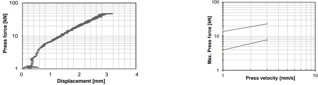
**Figure 2.** Experimental data of press rheology investigations for GMT material with a thickness of 4.2 mm at 260 °C: Exemplary force-displacement curve (left) at speed 1 mm/s and analysis approach for estimation of flow exponent (right) for different process stages
