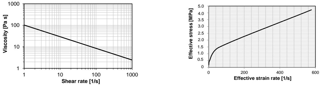
**Figure 3.** Results of the press rheology analysis for GMT material with 4.2 mm thickness at 260 °C: Viscosity curve (left) and estimated flow characteristics (right)
