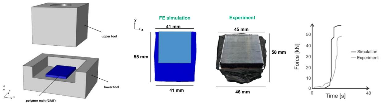
**Figure 4.** Numerical FE model for press rheology characterization test (left), numerical and experimental pressed polymer melt of rheology test with punch displacement 3 mm (middle) and force time curves of FE simulation and experimental investigation (right)
