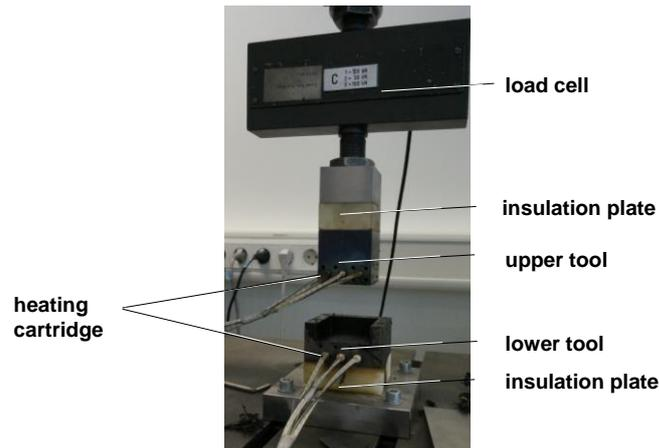
**Figure 1.** Experimental set-up for rheology investigations of GMT material
