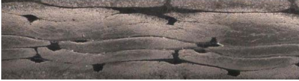
Figure 1. Perpendicular cross-section of UD NCF laminate, presenting fibre waviness [6].
