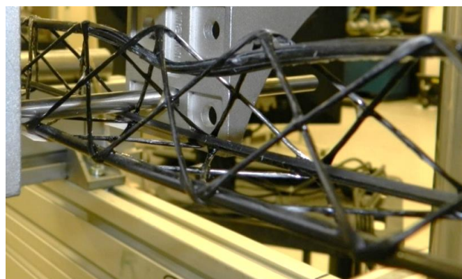
Figure 11. Tested sample showing debonding and failure of compression longitudinal member.
