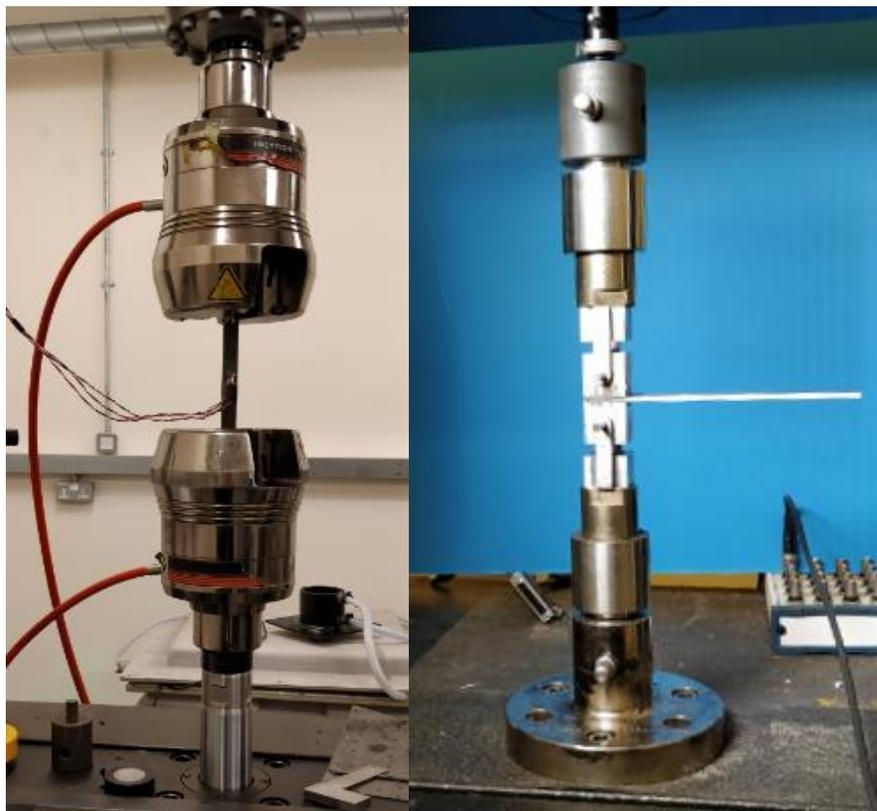
**Figure 1.** Tensile testing (left hand side) and Mode I delamination testing (right hand side) on Instron machine.
