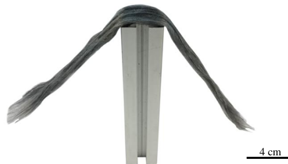
Figure 2: Sliver material, bending due to gravity shows low bending stiffness
