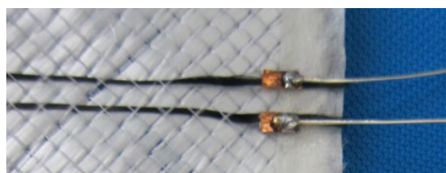
Figure 5. Exemplary electrical contacting of CFS onto textile reinforcement structure for further FRP applications before encircling isolation by heat shrink tubes
