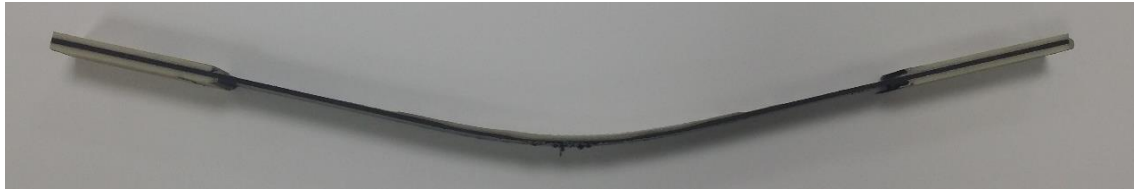
Figure 11. Excessive curvature in Fiberglass patch at 90°
