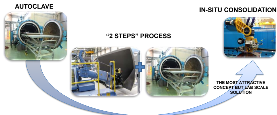
Figure .1 Evolution of automated lamination technologies: from the partial consolidation followed by autoclave or oven postconsolidation to the complete in-situ consolidation in one step.
