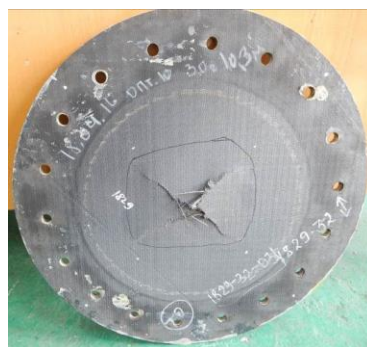
b) fiber rupture in several layers, at the back side ( Q=30 g, \beta=3.01 %, \delta=5.21 mm, m=7.91 \text{kg/m}^2 )
