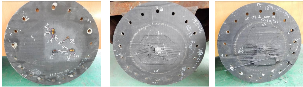
a) fiber rupture in the first layer, at the back side ( Q=20 g, \beta=1.84 %, \delta=5.75 mm, m=8.60 kg/m 2 ) b) fiber rupture in several layers, at the back side ( Q=45 g, \beta=4.15 %, \delta=5.76 mm, m=8.60 kg/m 2 ) c) penetration hole, back side ( Q=50 g, \beta=4.61 %, \delta=5.73 mm, m=8.60 kg/m 2 )
