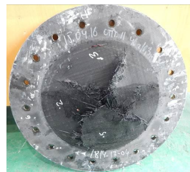
c) penetration hole, back side ( Q=40 g, \beta=3.55 %, \delta=5.88 mm, m=8.93 \text{kg/m}^2 )
