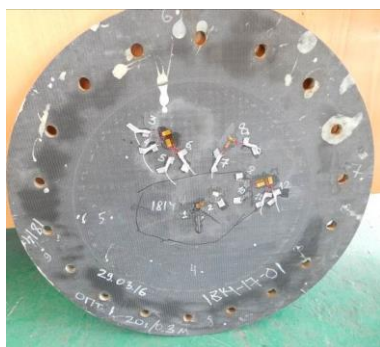
a) fiber rupture in the first layer, at the back side ( Q=20 g, \beta=1.78 %, \delta=5.94 mm, m=8.93 \text{kg/m}^2 )
