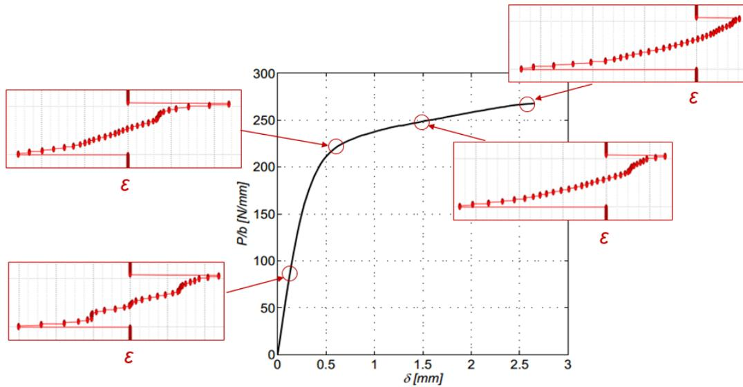
**Figure 1.** Load-displacement evolution in the central cross-section (in black) [3]. Normal strain profiles of the central cross-section at different moments of test (in red).
