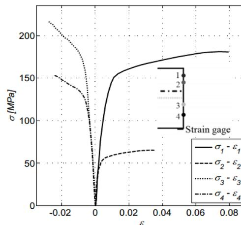
**Figure 2.** Stress-Strain evolutions at four different heights of a vertical central path [3].
