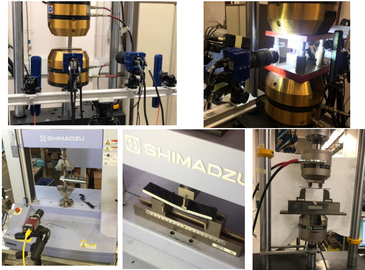
Figure 4. Characterisation test setups used, showing tensile (top left); compression (top right); Mode I (bottom left); Mode II (bottom middle); and; flexure (bottom right).
