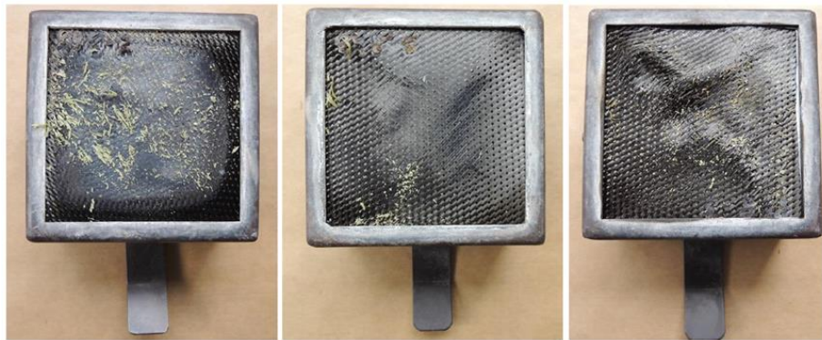
Figure 6. T650/NEXIMID ® MHT-R specimens (100×100 mm) after exposure to 70 kW/m 2 heat flux.
