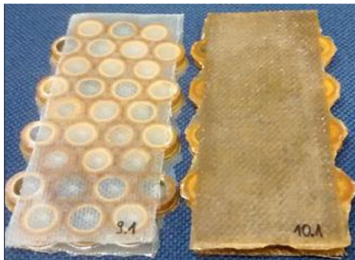
Figure 1. COMBOO structure – bamboo rings with glass fibers (left) and flax fibers (right)
