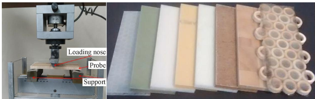
Figure 3. 3-Point bending setup and test specimen
