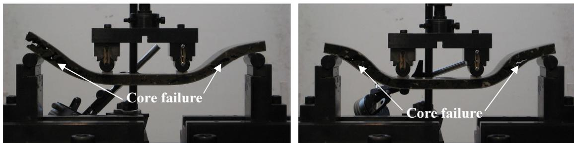
**Figure 3.** Four-point bending in third-point loading configuration, after core shear failure for BEC (left) and modified BEC (right) based sandwich structures.
