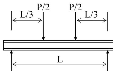
**Figure 1.** Third-point loading configuration in four-point bending test.
