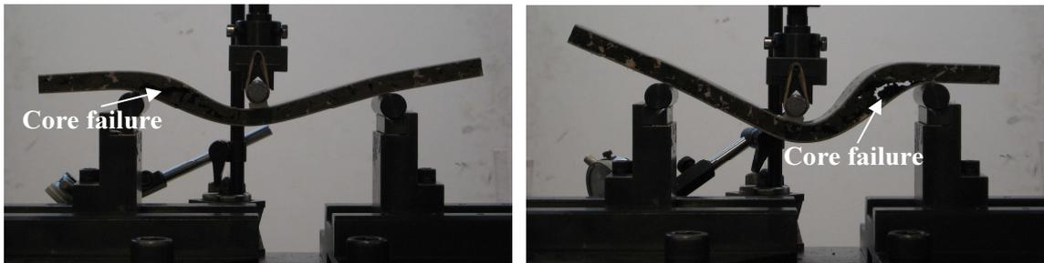
**Figure 2.** Three-point bending tests after core shear failure for neat BEC (left) and modified BEC (right) based sandwich structures.
