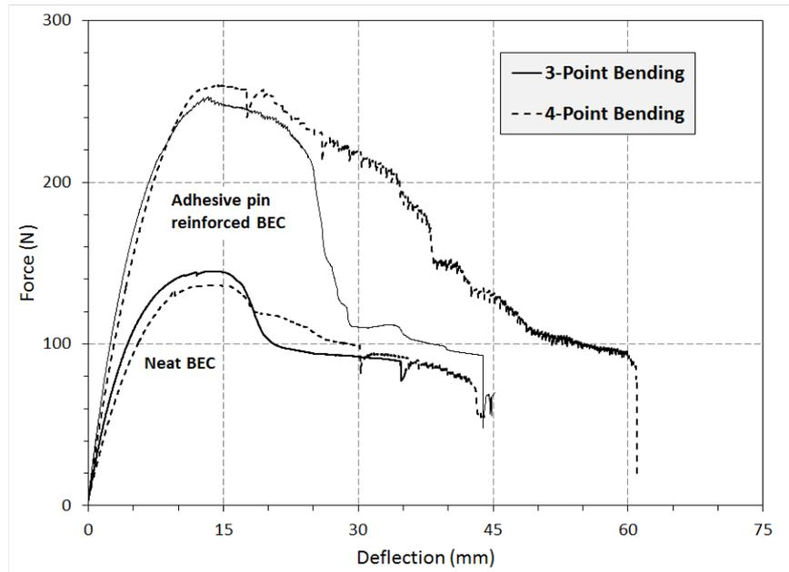
**Figure 4.** Load vs. deflection curves from three-point and four-point bending tests of representative sandwich structure specimens with both BEC based cores.
