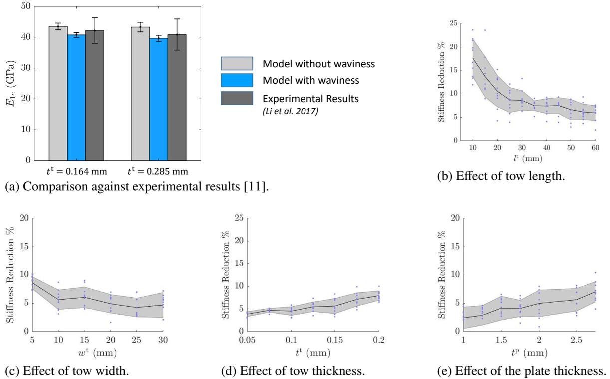
**Figure 2.** Parametric study of the effect of tow geometry on the in-plane stiffness reduction, and validation against experimental results.
