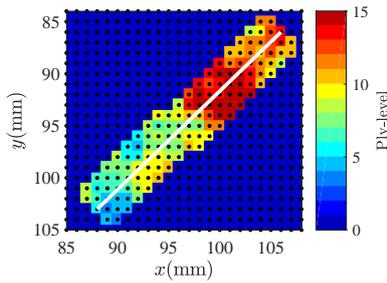
(a) Grid point mapping with  $s_{\text{grid}} = 1\text{mm}$ .
