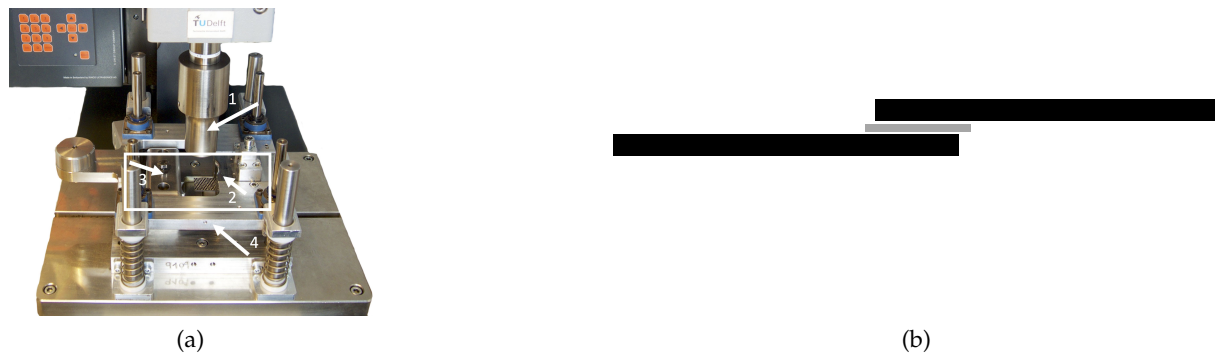
Figure 2: (a) In-house built welding jig and ultrasonic welding machine, (1) sonotrode, (2) upper coupon clamp, (3) lower coupon clamp, and (4) spring-supported platform for the upper clamp. The white box shows the location and orientation of the lap shear coupons schematically shown in (b). (b) CF/PPS coupons (black) and ED (grey).
