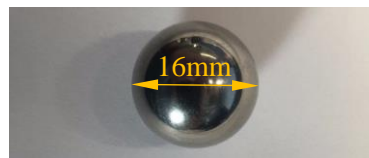
Figure 3. The 16mm diameter spherical AISI 52100 alloy stainless steel projectile
