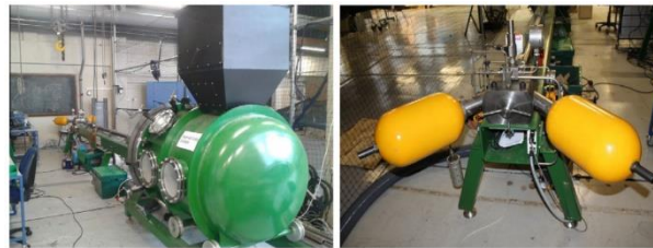
Figure 4. Imperial College gas gun; capture chamber (left) and breech (right) [7]
