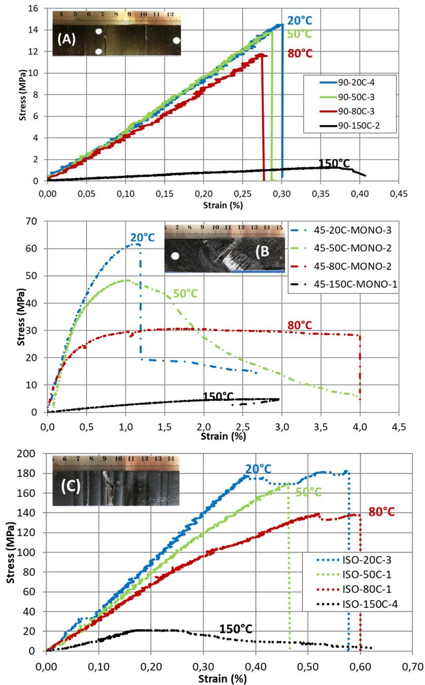
Figure 2 : Tensile stress-strain curves of samples (EC90 (A), EC45 (B) and ECiso (C)) submitted to homogeneous temperatures (20°C, 50°C, 80°C & 150°C) and mechanical loading until rupture
