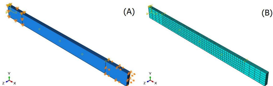
Figure 4 : Modelling of sample EC45 by FEA; (A) and Boundary condition. (B) Mesh of structure of sample EC45.
