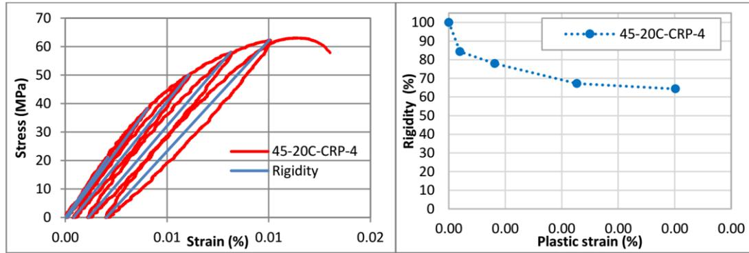
Figure 3 : Tensile test for EC45: Cyclic loading, Shear evolution vs. Plastic strain
