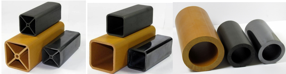
Figure 2. Different profile geometries, green bodies (ochre coloured), porous C-templates (lying on top, right picture: in between) and C/Si/SiC-ceramics (right side).
