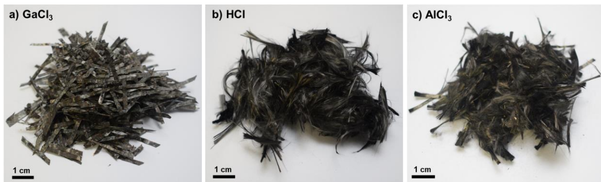
Figure 2. Recycled carbon fibers obtained by vaporsolvvolysis using as catalyst a) \text{GaCl}_3 , b) \text{HCl} , and c) \text{AlCl}_3 .
