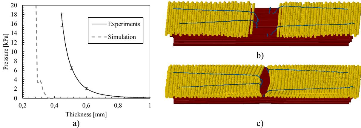
**Figure 5.** Comparison of the experimental and virtual compaction characterization a), and simulation results at 38% FVF b) and 67% FVF c).
