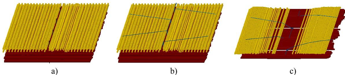
**Figure 3.** a) Penetration of the fiber bed, b) idealization of the stitching yarn geometry, c) and simulation result after the pretension of the stitching yarns.
