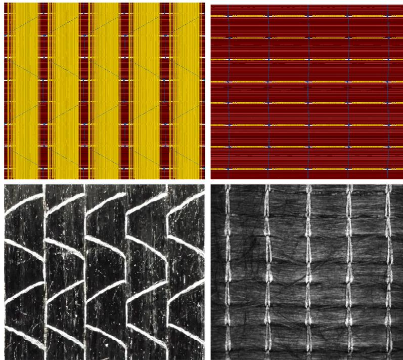
**Figure 4.** Comparison of the virtual “as-manufactured” geometry (top) and the studied non-crimp fabric (bottom).
