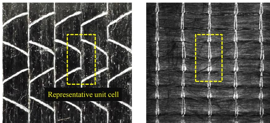
**Figure 1.** Illustration of the representative unit cell on the front face (left) and back face (right) of the  $0^\circ/90^\circ$  biaxial tricot-chain stitched NCF.
