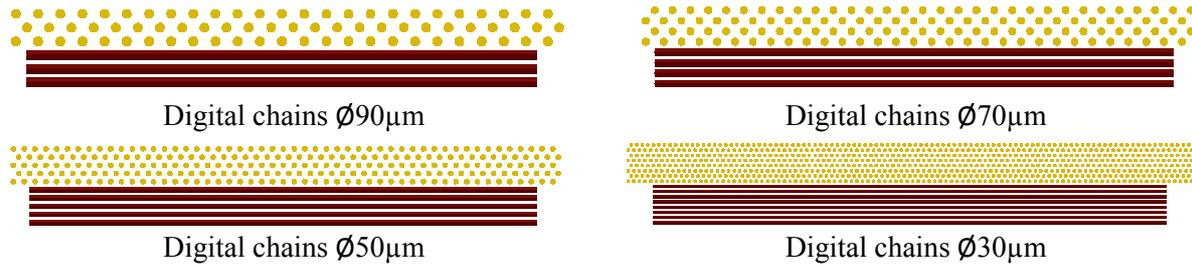
**Figure 2.** Model of the fibrous mat for various tow discretization with constant fiber volume fraction.
