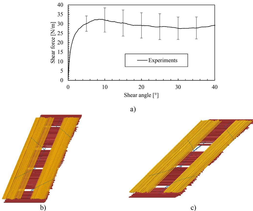
**Figure 6.** Experimental results of the picture frame shear tests a), and simulation results at 22.5° b) and 45° c) shear angle.
