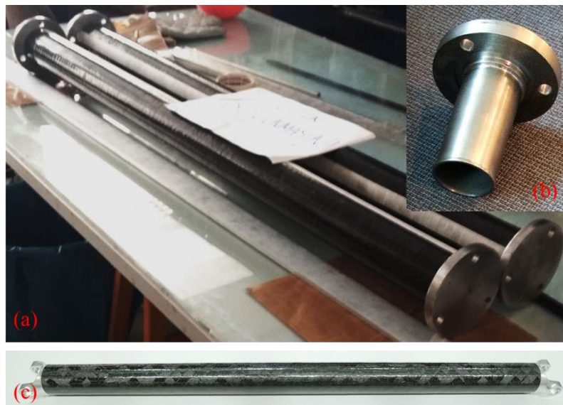
Figure 2. (a) the composite shaft manufactured, (b) insert for testing, (c) final assembly with regular yokes.
