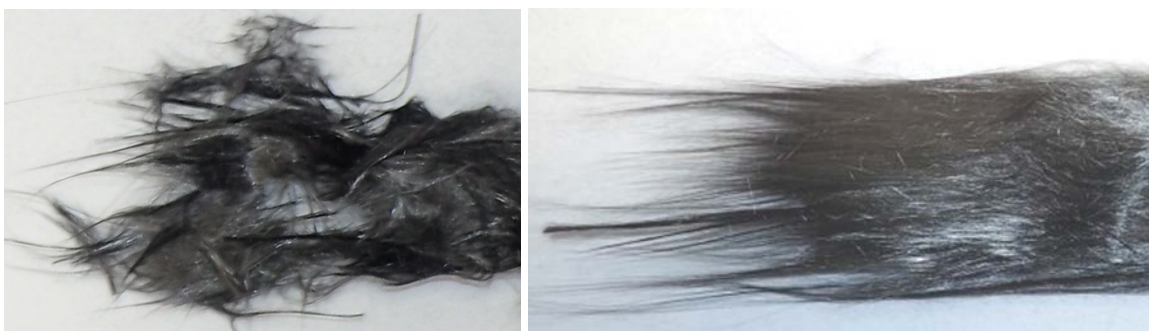
Figure 5. Left: rCF sliver from roller card, Right: High aligned rCF sliver after drawing
