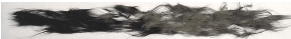
Figure 6. Poorly oriented sliver due to too high draft
