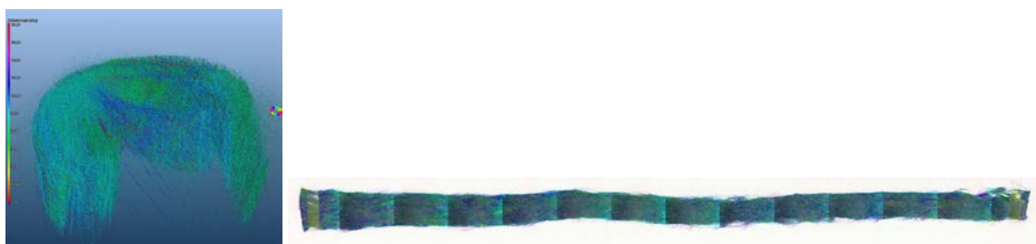
Figure 8. CT scan (left) 2,5 x 1 cm 2 compared to POLKA measurement 100 x 9 cm 2 (right)
