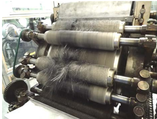
Figure 3. Exemplary a roller card with flexible wires processing LrCF of the DITF
