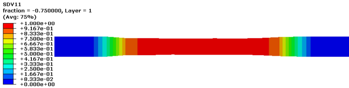
Figure 3. Localization of damage ( d_{12} ) in test specimen – shear test.
