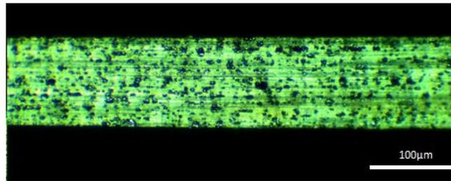
**Figure 2.** Example of a good speckle pattern on a hemp fibre.
