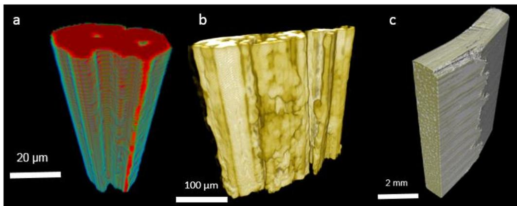
**Figure 1.** Three-dimensional reconstructions of an elementary fibre (a) and a technical fibre (b) of hemp. A typical hemp fibre reinforced composite sample undergoing deformation (3 point bending test) (c).
