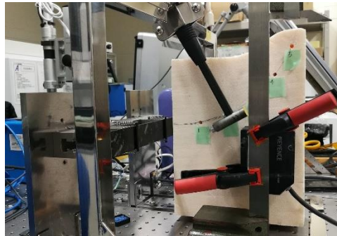
Figure 3. Lateral impact equipment
