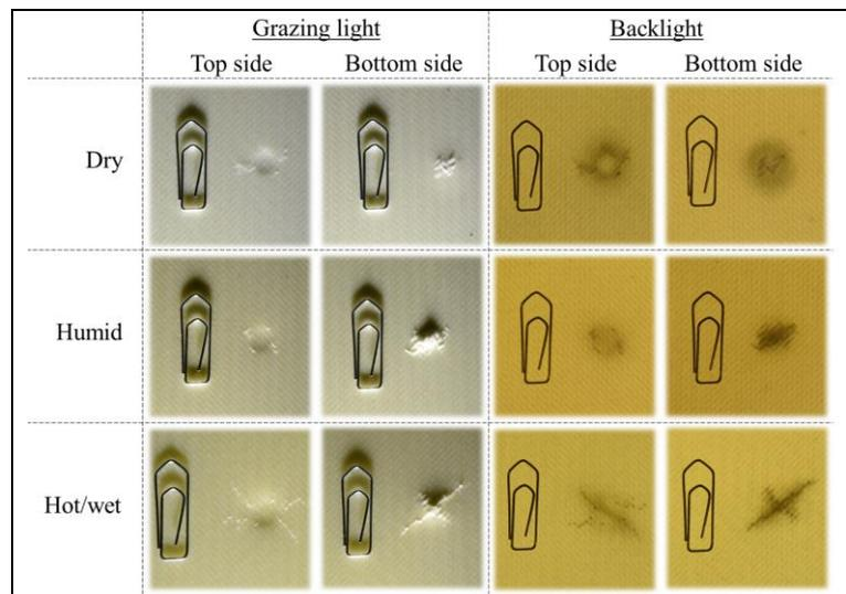
**Figure 3:** Comparison of visual surface damages in grazing light (left) and damaged areas by means of backlight analyses (right). All displayed specimens were impacted with an impact energy of 20 J.
