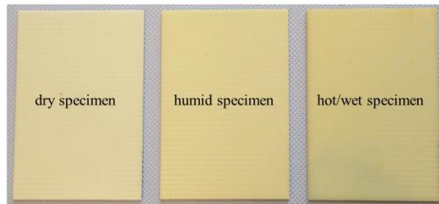
**Figure 1:** Surface discoloration of the specimens (size: 150 mm x 100 mm) after 623 h of conditioning.
