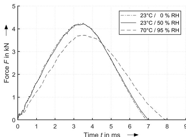
**Figure 5:** Exemplary force-time curves as a function of the specimen conditioning. All specimens were impacted with an impact energy of 12 J.
