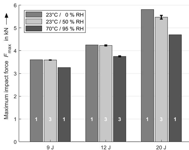
**Figure 6:** Maximum impact force (mean values) of all specimens as a function of the impact energy. The number of tested specimens is given within the bars, error bars are indicated when applicable (very little scatter).
