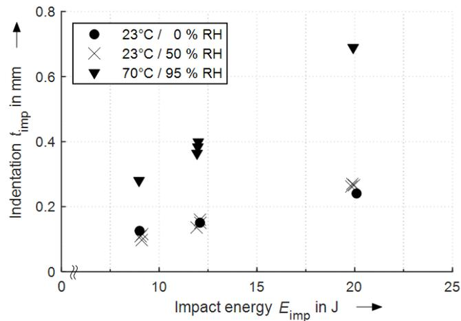
**Figure 4:** Impactor indentation  $t_{imp}$  as a function of the impact energy  $E_{imp}$ .
