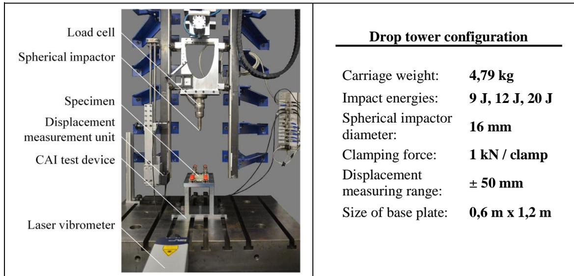
**Figure 2:** Left: Experimental set-up for low velocity impact tests. Right: Test rig configuration.
