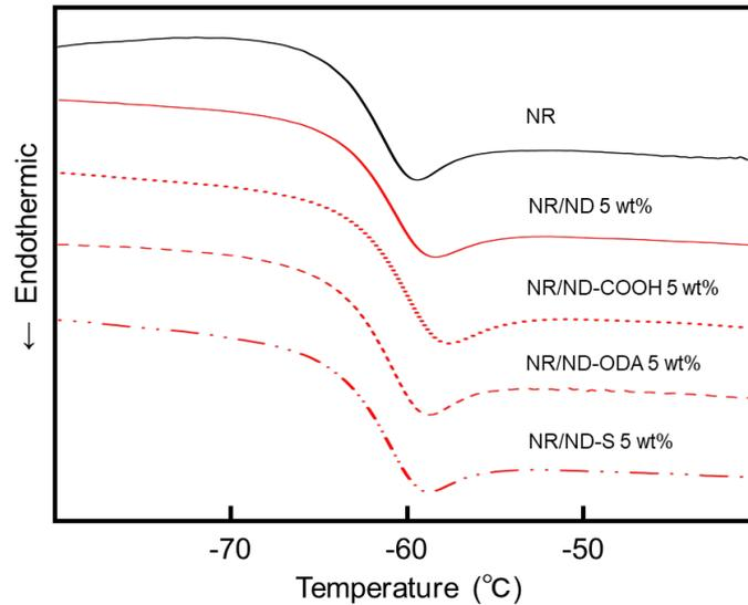
Figure 4. DSC curve of NR and NR / ND nanocomposites.
