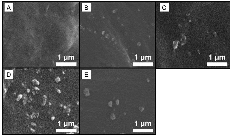
Figure 3. SEM images of NR (A), NR/ND (B), NR/ND-COOH (C), NR/ND-ODA (D) and NR/ND-S (E) nanocomposites (5 wt%).
