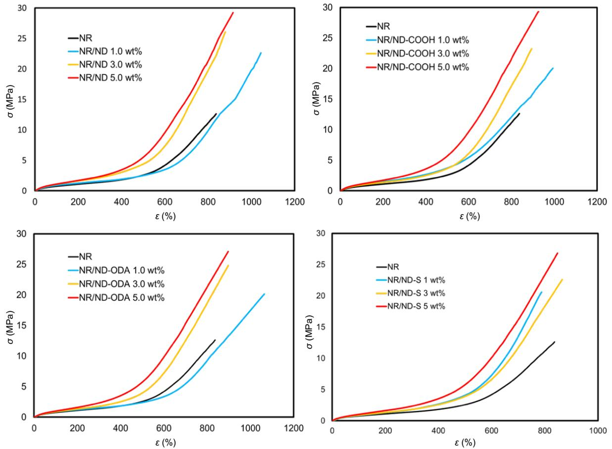
Figure 5. Stress-strain curves of NR and NR/ND nanocomposites.
