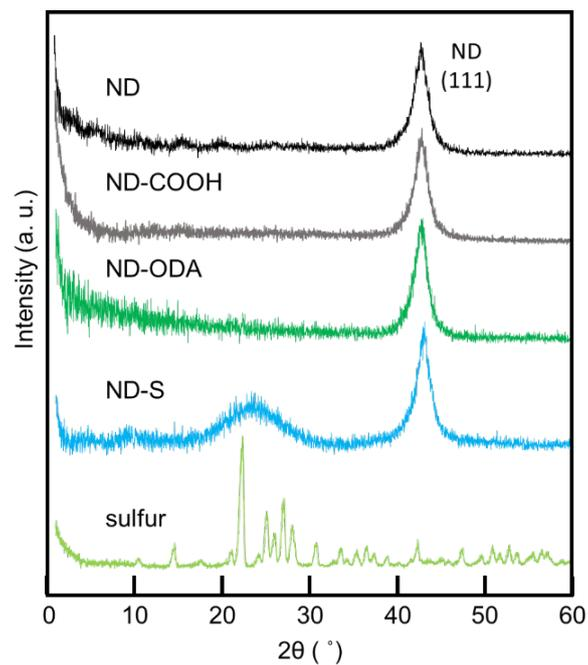
Figure 2. X-ray diffraction profiles of ND, ND-S and sulfur.
