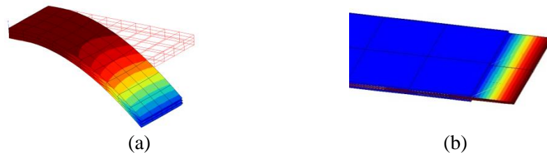
Figure 6. Simulation of the experimental out-of-plane bending (a) and inter-ply sliding (b) tests
