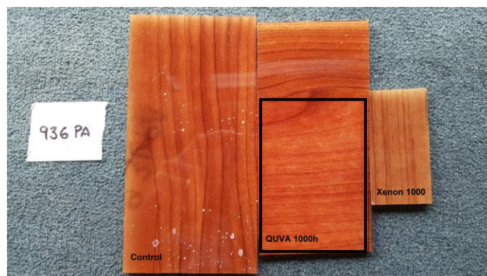
Figure 4. Resin 936PA sample after the accelerated weathering test
