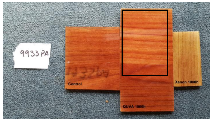
Figure 5. Resin 9933PA sample after the accelerated weathering test
