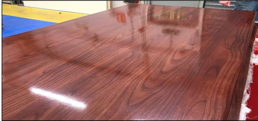
Figure 7. Moulded demonstrator in the as-released finish, showing the aesthetic quality possible using the wood effect polyester veil and novel high UV resistance resin
