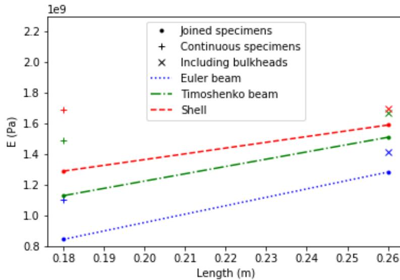
**Figure 3:** Quasi-static flexural modulus of the specimens, derived from the load-displacement curves using three different structural models, as a function of specimen length. Lines (dot markers) depict specimens with no bulkheads, produced by joining a number of segments (see Table 2). + markers depict specimens without any joining, whereas x markers depict specimens including bulkheads.
