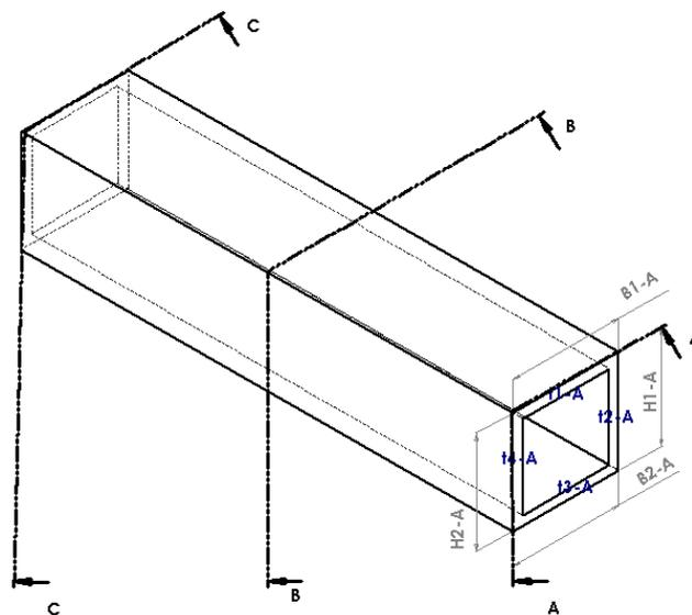
**Figure 1:** Depiction of the measurement points for each specimen segment. A, B and C denote the 3 sections where measurements were obtained. H, B and t represent measurements of height, breadth and thickness, respectively. No thickness measurements were obtained at the midpoint.
