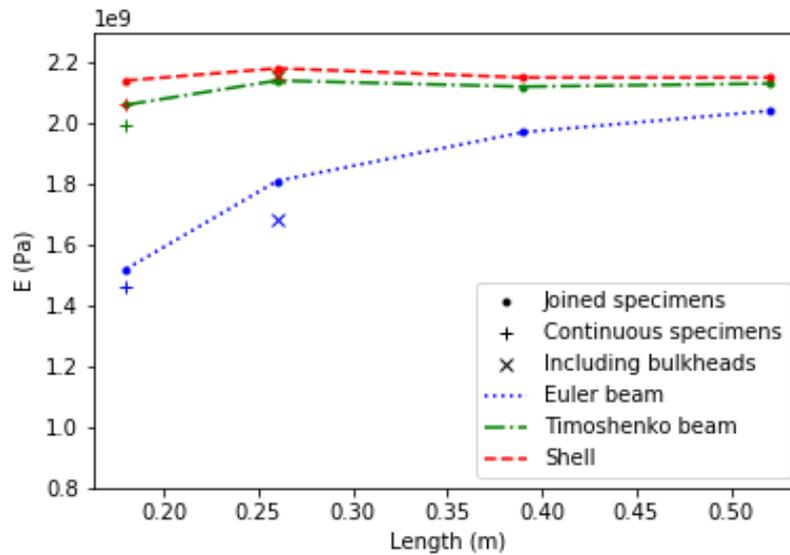
**Figure 2:** Dynamic flexural modulus of the specimens, derived from the 2-node bending natural frequency using three different structural models, as a function of specimen length. Lines (dot markers) depict specimens with no bulkheads, produced by joining a number of segments (see Table 2). + markers depict specimens without any joining, whereas x markers depict specimens including bulkheads.
