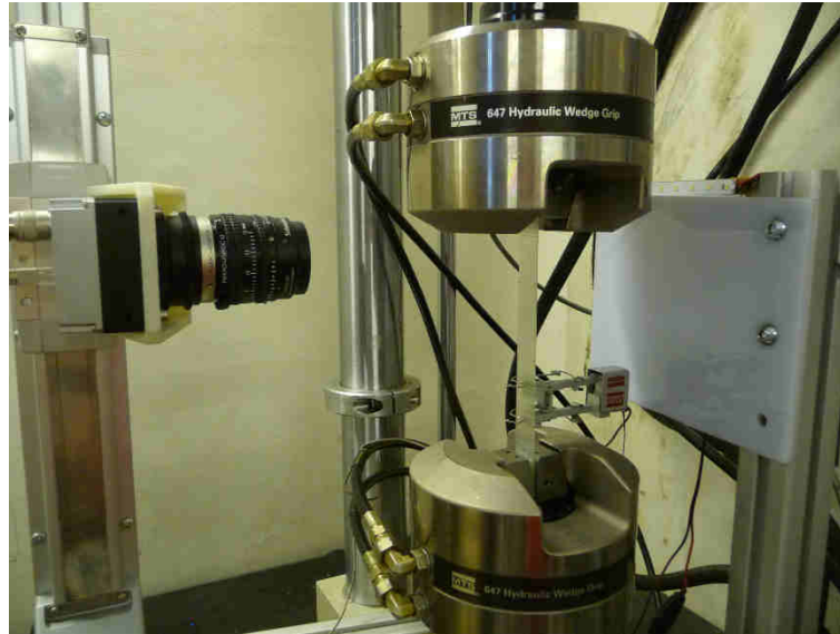
Figure 2. Experimental test setup. A linear camera is mounted in front of the specimen and a light source is placed behind it to monitor the transverse crack evolution during the tests [12].
