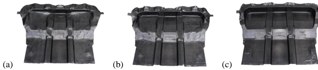
Figure 8. Forming study results for residual mold travel of 70mm (a), 40mm (b) and 25mm (c).
