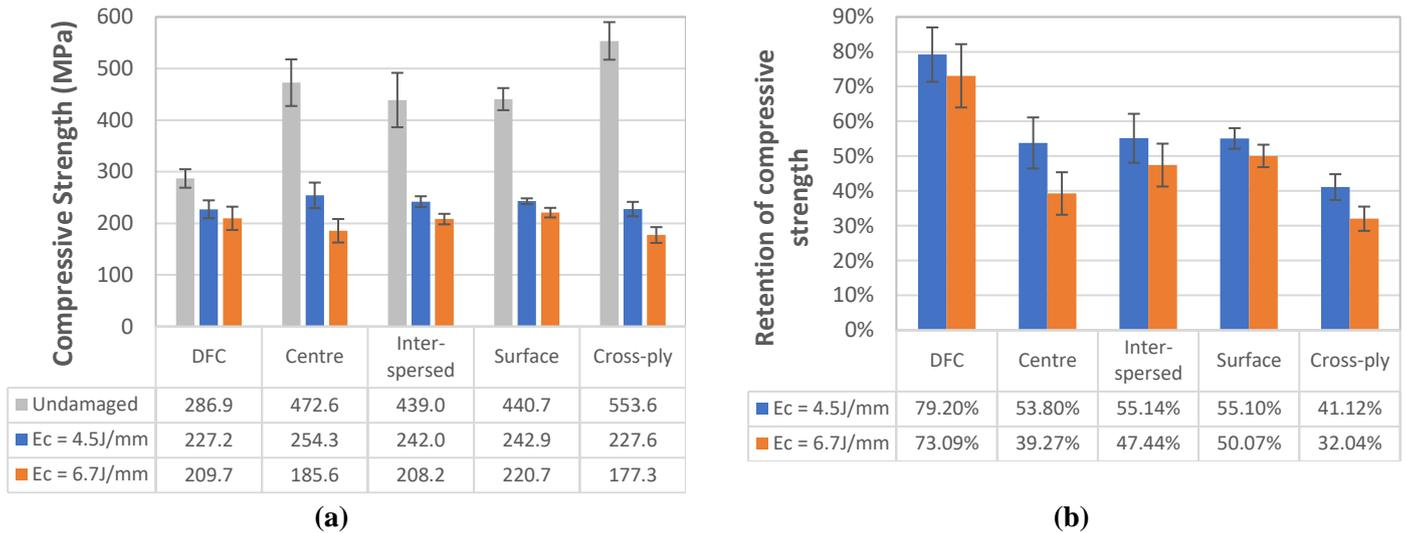
**Figure 14.** Compressive strengths of each fibre architecture prior to impact testing and after exhibiting target out-of-plane impacts of 4.5J/mm and 6.7J/mm (a) and the percentage of retained compressive strength for each impact (b)
