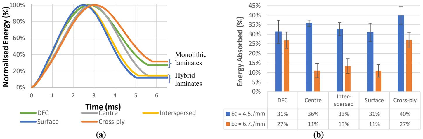
**Figure 3.** Typical impact energies with respects to time during a 6.7J/mm impact, normalised by dividing by the peak impact energy of each impact (a). Selected examples are the closest results to average results shown in (b).
