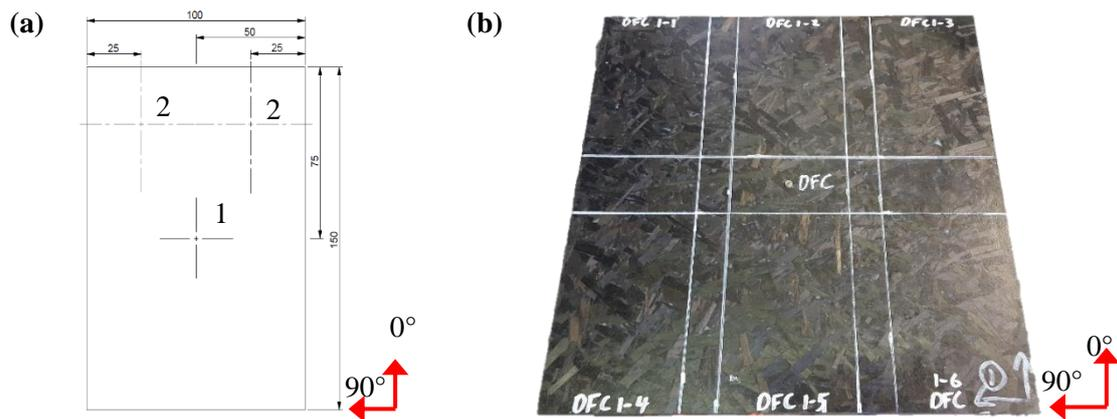
*Figure 2. Drop weight and CAI specimen dimensions with the position of the impactor, location 1, and the strain gauges, location 2, (a) and the plaque cutting plan (b)*
