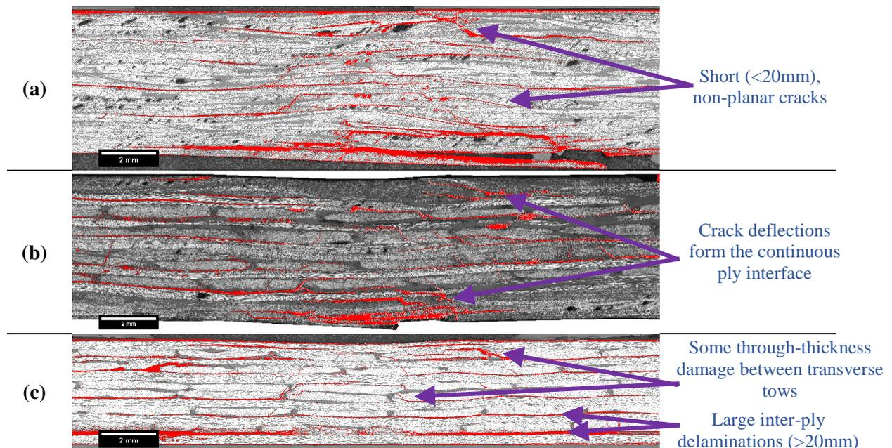
**Figure 6.** Micrographs of impacted specimens with a threshold applied to show damage ( $J_c = 6.7\text{J/mm}$ ). (a) DFC specimen, (b) Hybrid with NCF plies Intersperse and (c) Cross-ply. The middle of the image is aligned with the out-of-plane impact location.
