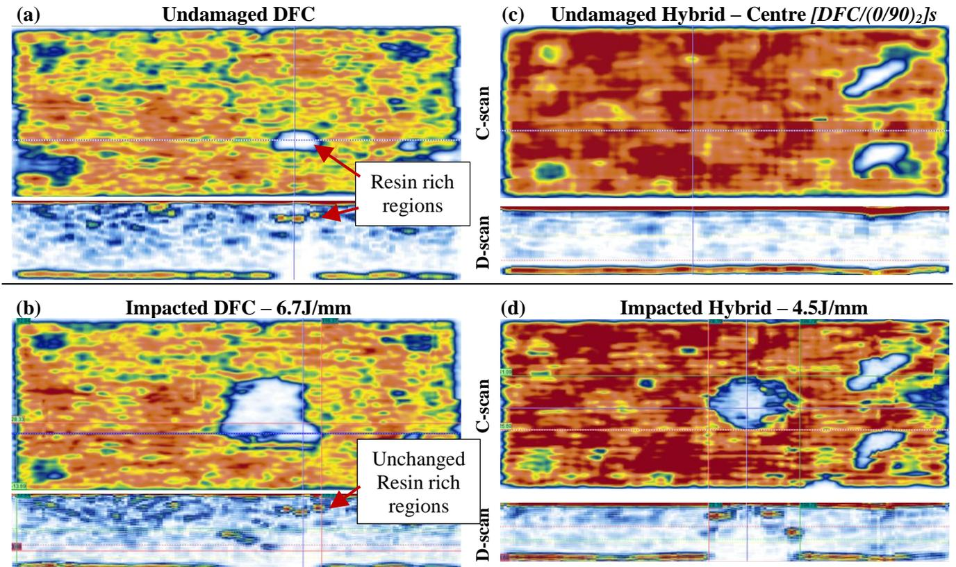
**Figure 4.** Ultrasonic C-scans and D-scans of a DFC specimen: (a) undamaged and (b) impacted ( $E_c = 6.7\text{J/mm}$ ), and of a Hybrid specimen (continuous material positioned at the centre): (c) undamaged and (d) impacted ( $E_c = 4.5\text{J/mm}$ ).
