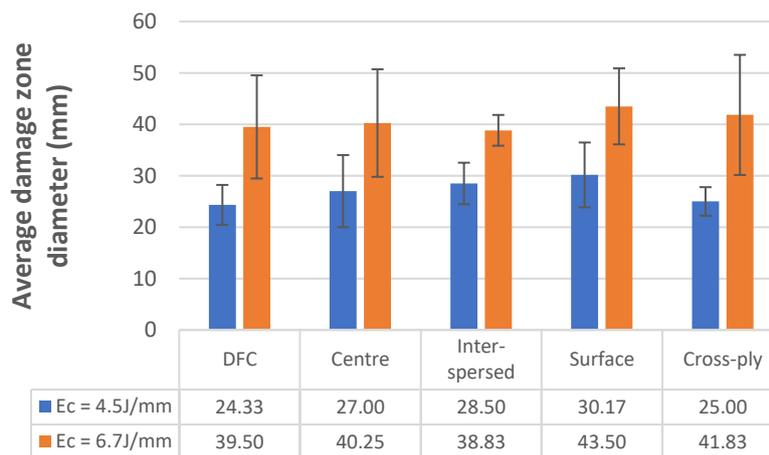
**Figure 5.** Average damage zone diameters determined by the length and width of damage zones measured from each C-scan
