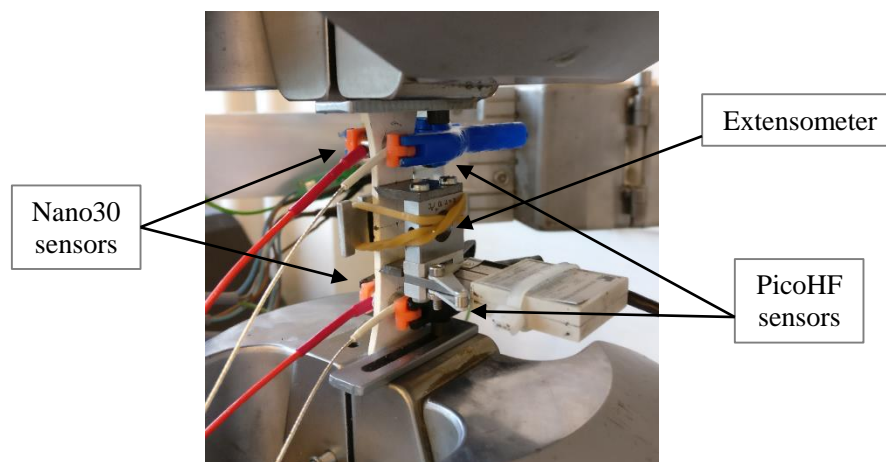
Figure 2. Multi-sensor AE monitoring during macroscopic tensile test
