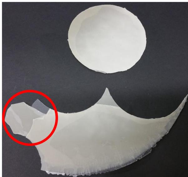
**Figure 1.** Image of the delamination of the PLA laminated composites containing 100 wt.% NFC papers as reinforcement.
