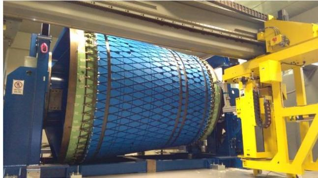
**Figure 13.** Winding of the grid structure of I/S 2-3 TM0
