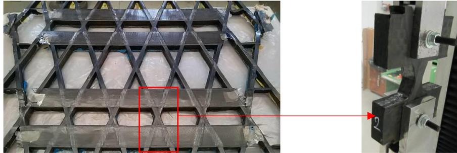
**Figure 8.** Type IV panels and end ring sub-components testing
