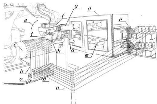
**Figure 4.** Patented technique to interlace the grid structure ribs (helixes) and hoop
