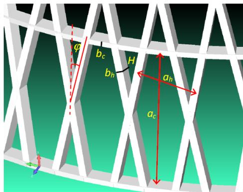
**Figure 1.** Typical design parameters of a grid structure.
