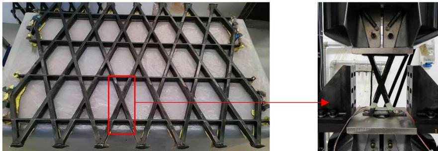
**Figure 7.** Type III panels and Clepsydra sub-components testing
