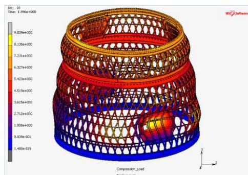
**Figure 12.** Non-linear buckling analysis
