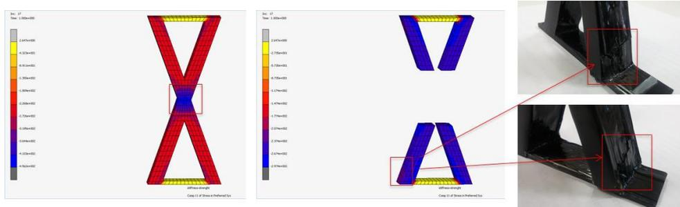
**Figure 10.** Comparison between FEM simulation and experimental results
