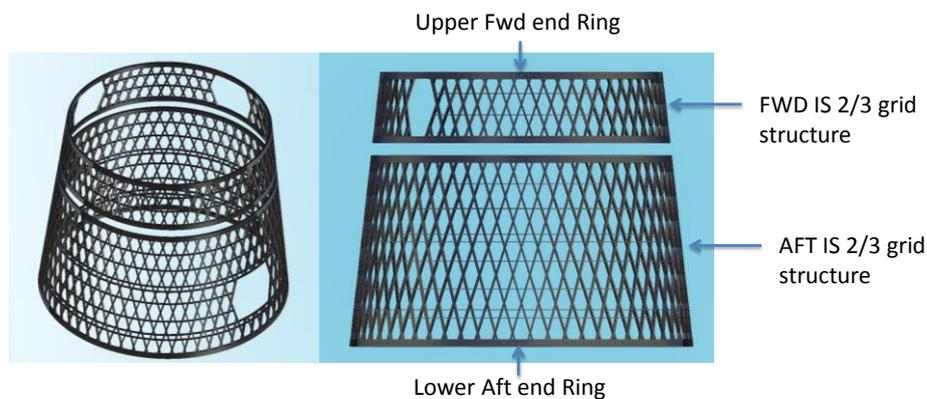
**Figure 3.** I/S 2-3 grid structure layout
