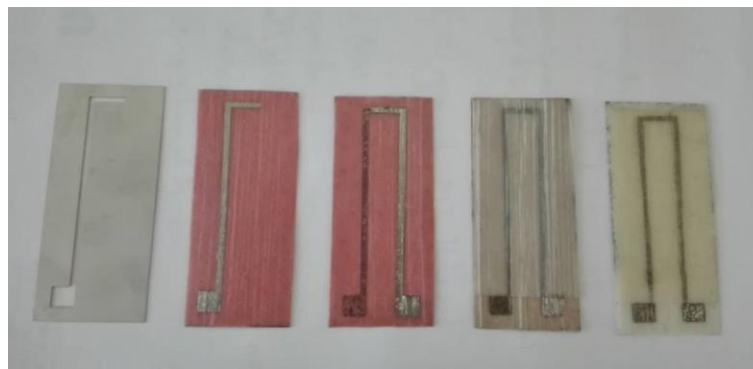
Figure 5. The different steps in embedding a thin film thermocouple in a composite prepreg lay-up. From left to right: the sputter mask, a first leg of constantan, a second leg of chromel, embedding the TFTC in the lay-up and finally a cured composite. The release foil has a pink color.
