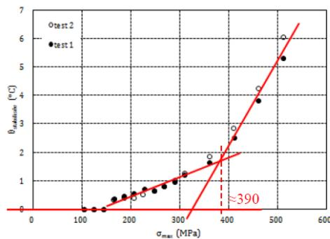
**Figure 12** : Self-heating curve obtained by [23] on woven carbon/thermoplastic composite
