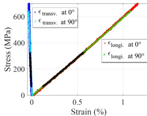
**Figure 6 :** Stress-strain curve, for the longitudinal and transversal strains for samples at  $0^\circ$  and  $90^\circ$ , and the domains used for the evaluation of the Young modulus and the Poisson's ratio (black)
