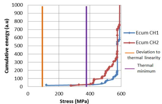
**Figure 11** : Cumulative energy measured by two acoustic sensors during a quasi-static tensile test
