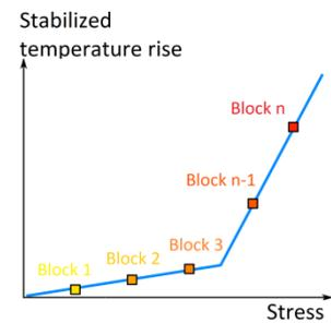
**Figure 3** : Self-heating curve
