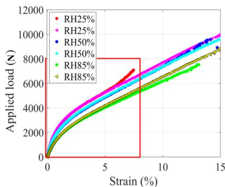
**Figure 4** : Stress-strain curves for specimens oriented at 45°, with two samples tested per humidity level
