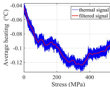
**Figure 8** : Gaussian filtering of the thermal signal
