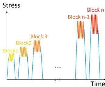
**Figure 1** : Schematic representation of self-heating tests
