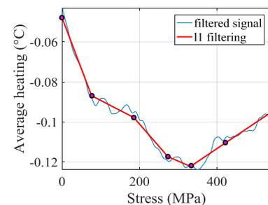
**Figure 9** : Application of the  $l_1$  trend filtering on the filtered signal
