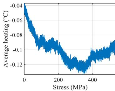
**Figure 7** : Evolution of the spatial average heating of the sample with the stress during a static test
