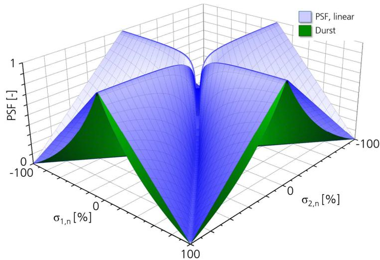
**Figure 5.** Principal stress factor *PSF* over normalized principal stresses in a shell element compared to Durst’s anisotropy value.
