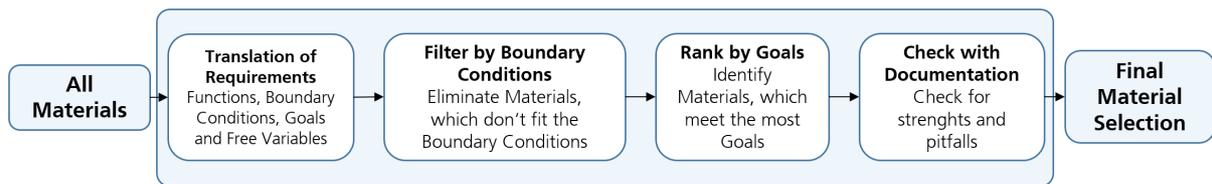
**Figure 1.** The four-levelled process of strategic material selection (reprod. from [8]).
