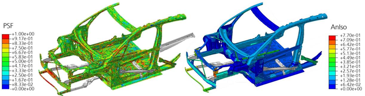
**Figure 8.** Plot of the element-wise *PSF* (left) and the component-wise *AnIso* (right) for a section of the automotive *BIW* based on the superposition of a full overlap frontal barrier crash and a pole side impact.
