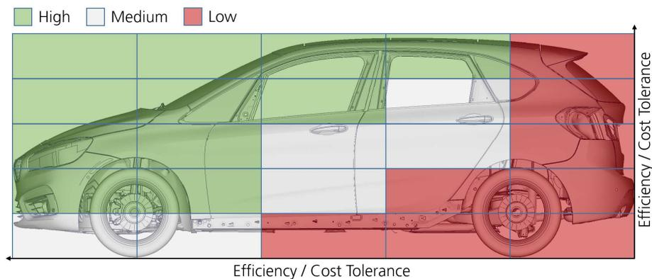
**Figure 11.** Qualitative distribution of the efficiency of lightweight design measures and related cost tolerance along the longitudinal and vertical axes of a vehicle with a front engine (reprod. from [28]).
