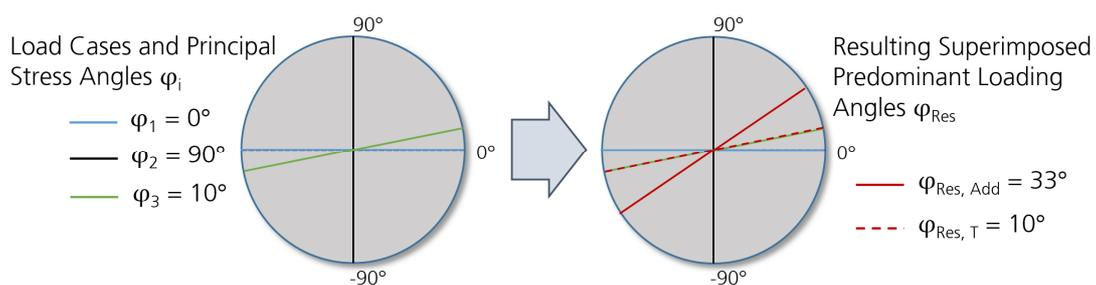
**Figure 6.** Comparison of the resulting loading directions for superimposed load cases from computing the arithmetic mean and from applying the proposed tensor addition technique.
