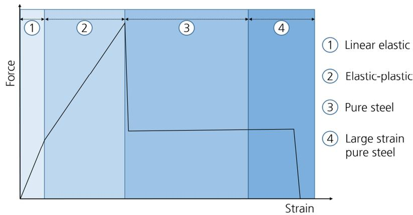
**Figure 12.** Schematic depiction of the force-strain-behavior of composite-metal-hybrid material systems in a tensile test.
