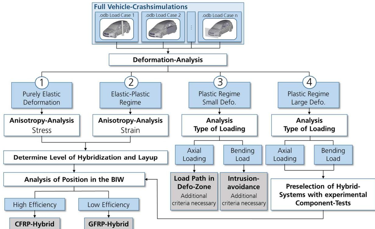
**Figure 13.** Systematic evaluation process to assess the suitability of composite-metal-hybrid materials systems based on the criteria proposed.
