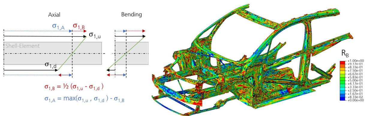
**Figure 10.** Relation of the first principal stresses on the upside and downside of shell element for a rather axially an rather transversely loaded case (left) and the evaluation of the ratio of bending load  $R_B$  in the *BIW* for a frontal barrier crash with 40 % overlap (right).
