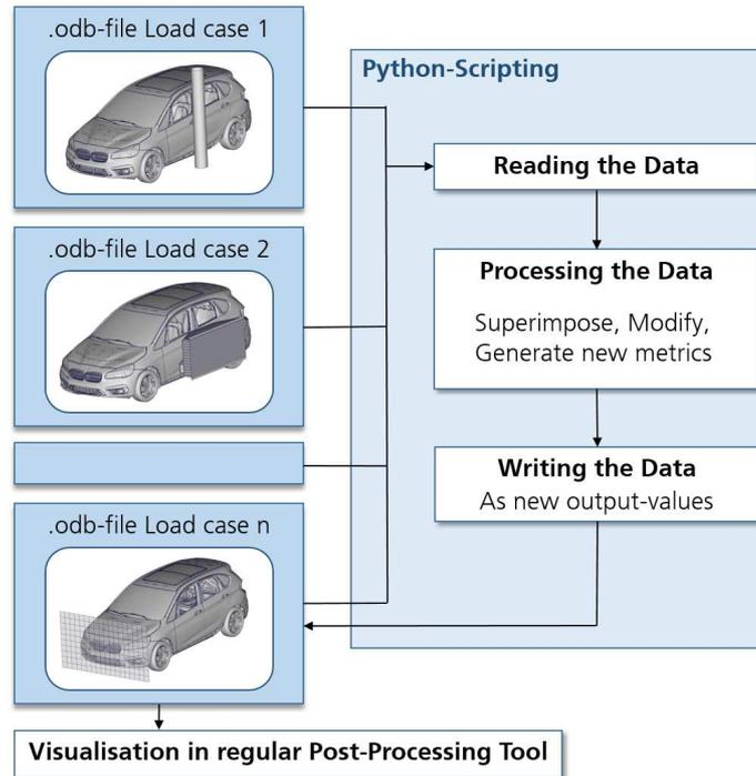
**Figure 4.** Schematic depiction of the technical workflow of the loading analysis.
