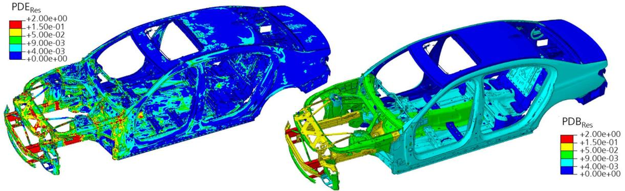
**Figure 9.** Plot of the element-wise  $PDE_{Res}$  (left) and the component-wise  $PDB_{Res}$  (right) indices for the superimposed maximum plastic deformation for two frontal crash load cases with different overlap.
