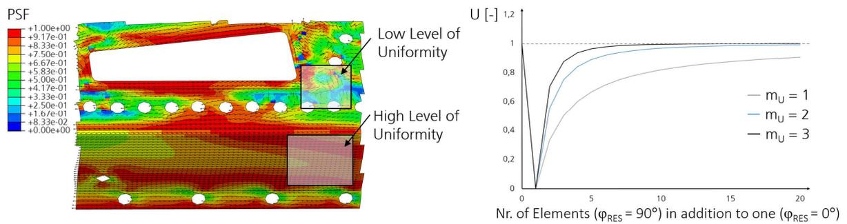
**Figure 7.** Elementwise plot of the *PSF* in a door sill section with resulting predominant loading directions showing areas of high and low levels of directional uniformity (left) and effect of the exponent  $m_U$  on the convergence of the uniformity index  $U$  with respect to the distribution of local resulting loading directions (right).
