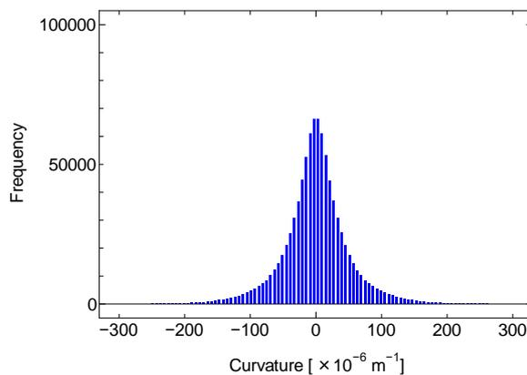
**Figure 2.** A histogram of the simulated curvatures generated by the thermal deformation of the CFRP plate due to fiber orientation errors (target stacking sequence:  $[0_2/-45_2/90_2/45_2]_s$ ).
