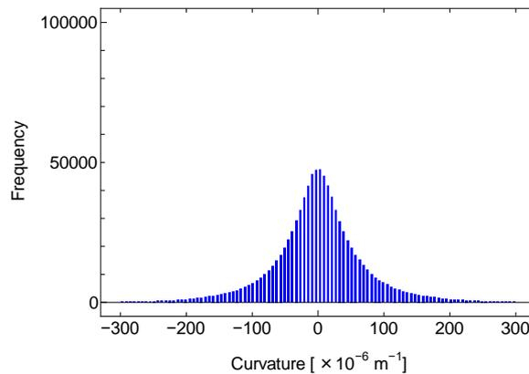
**Figure 1.** A histogram of the simulated curvatures generated by the thermal deformation of the CFRP plate due to fiber orientation errors (target stacking sequence:  $[0/-45/90/45]_s$ ).
