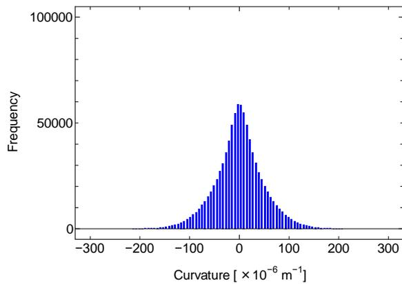
**Figure 4.** A histogram of the simulated curvatures generated by the thermal deformation of the CFRP plate with the optimized target stacking sequence due to fiber orientation errors (target stacking sequence:  $[0/-47/71.5/5]_s$ ).
