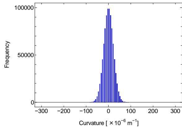
**Figure 5.** A histogram of the simulated curvatures generated by the thermal deformation of the CFRP plate with the optimized target stacking sequence due to fiber orientation errors (target stacking sequence:  $[0/-65/59.5/58/-46/-45/56/4]_s$ ).
