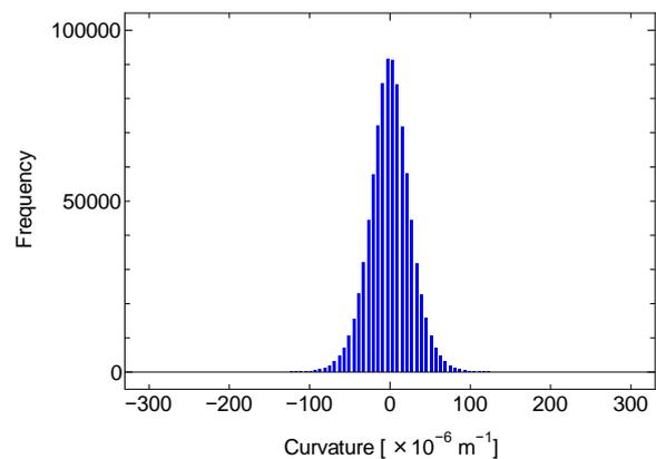
**Figure 3.** A histogram of the simulated curvatures generated by the thermal deformation of the CFRP plate due to fiber orientation errors (target stacking sequence:  $[0/-45/90/45]_{2s}$ ).
