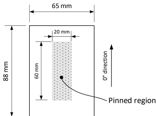
**Figure 1.** Geometry of Z-pinned samples
