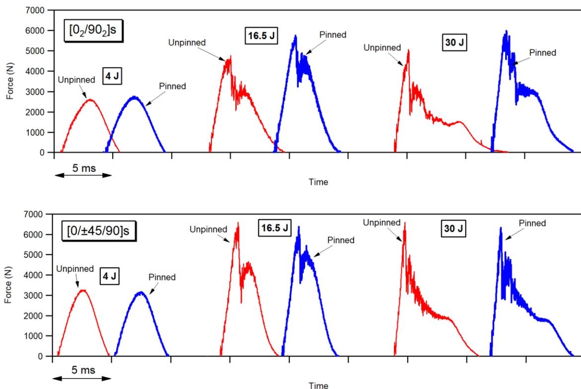
**Figure 2.** Force-time histories measured during impact events on unpinned and pinned samples
