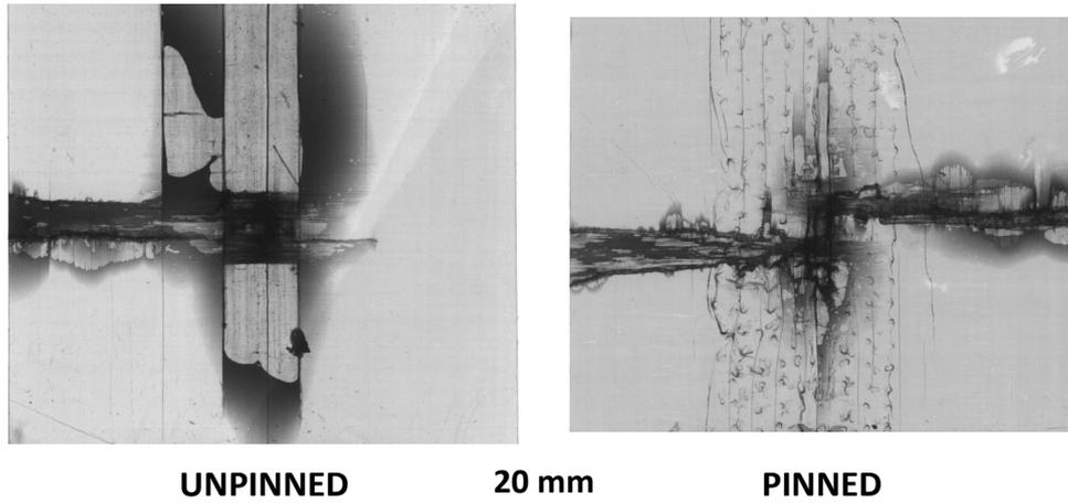
**Figure 6.** X-radiographs of damage after CAI testing in unpinned and pinned  $[0_2/90_2]_s$  laminates impacted at 16.5 J.
