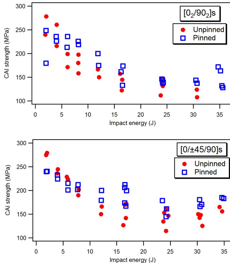
**Figure 5.** CAI strength vs impact energy of  $[0_2/90_2]_s$  and  $[0/\pm 45/90]_s$  impacted samples
