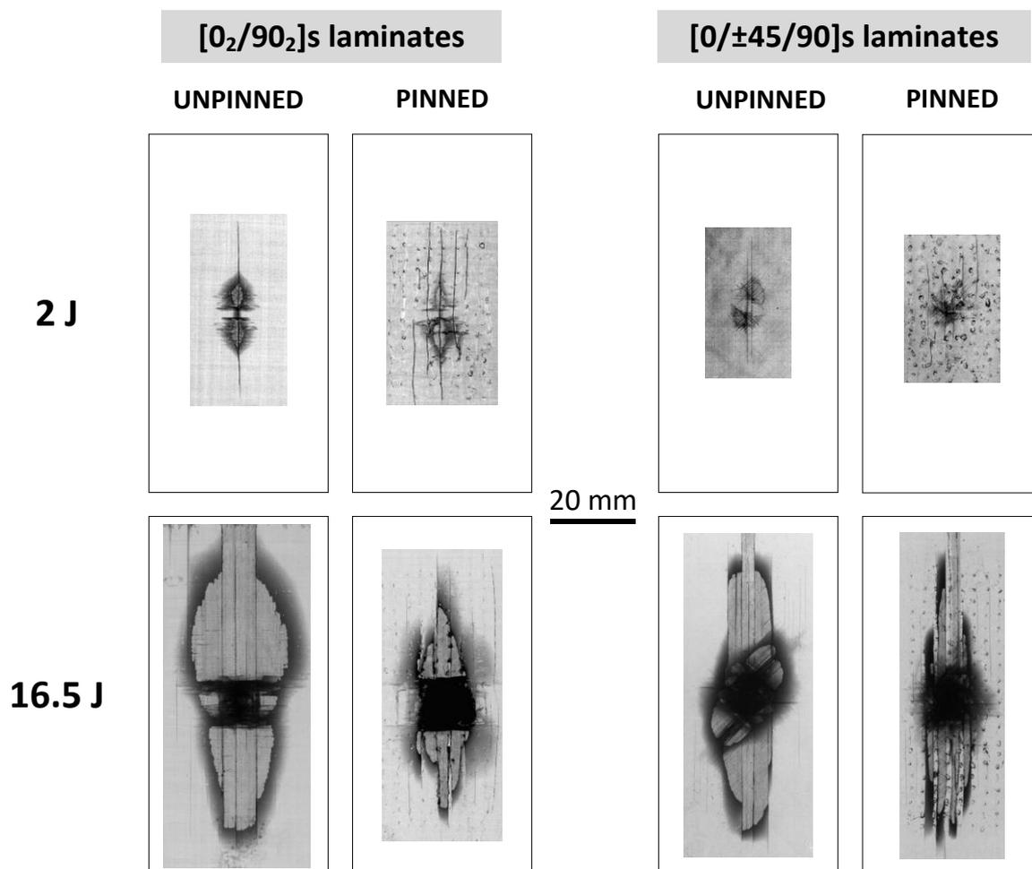
**Figure 3.** X-radiographs of impact damage in unpinned and pinned  $[0_2/90_2]_s$  and  $[0/\pm 45/90]_s$  laminates
