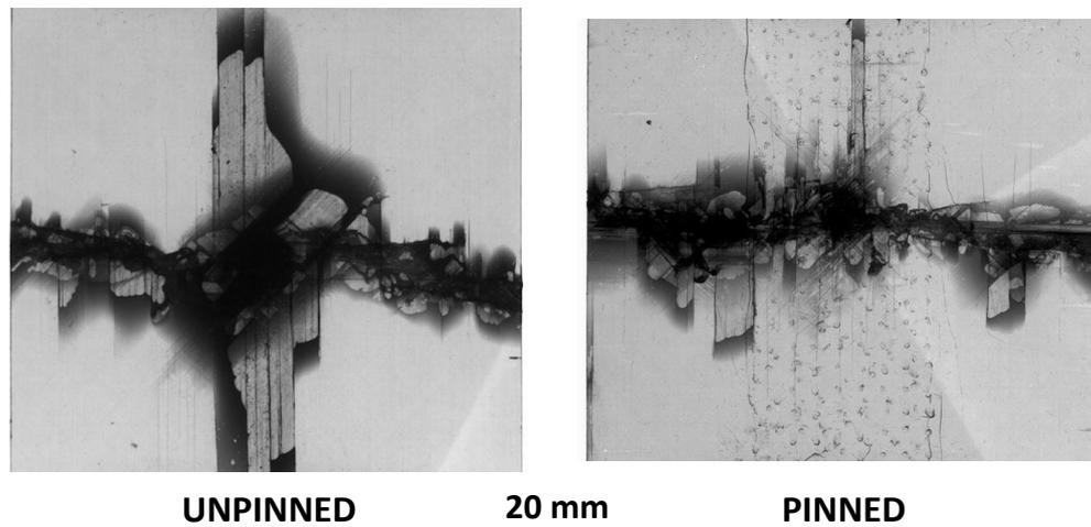
**Figure 7.** X-radiographs of damage after CAI testing in unpinned and pinned  $[0/\pm 45/90]_s$  laminates impacted at 16.5 J.
