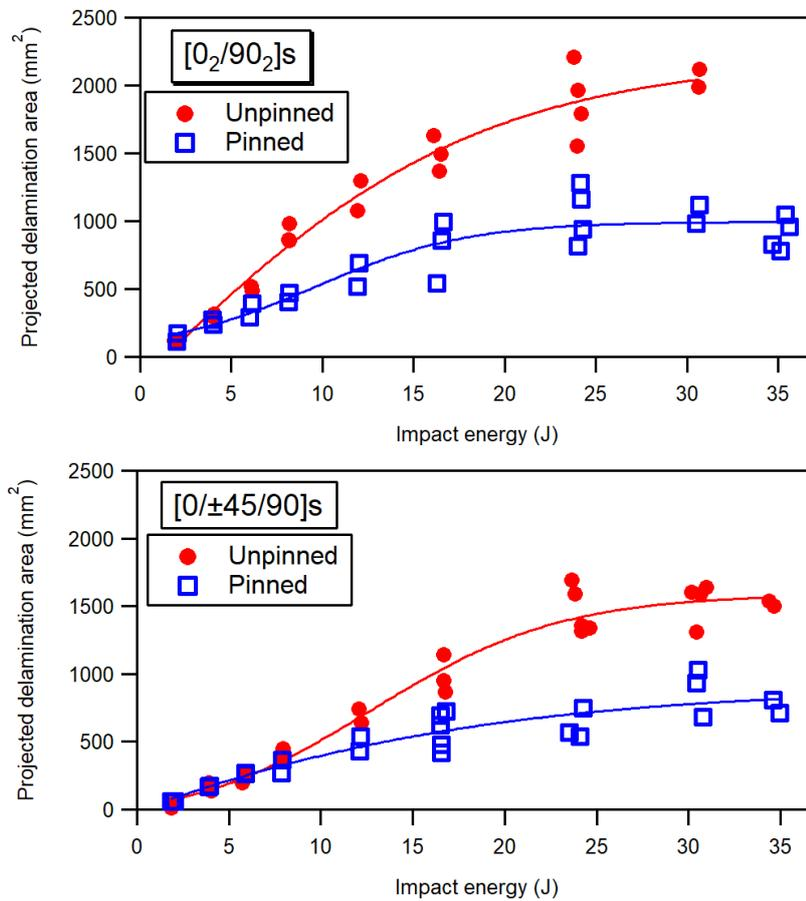
**Figure 4.** Damage area vs impact energy for unpinned and pinned [0<sub>2</sub>/90<sub>2</sub>]s and [0/±45/90]s laminates
