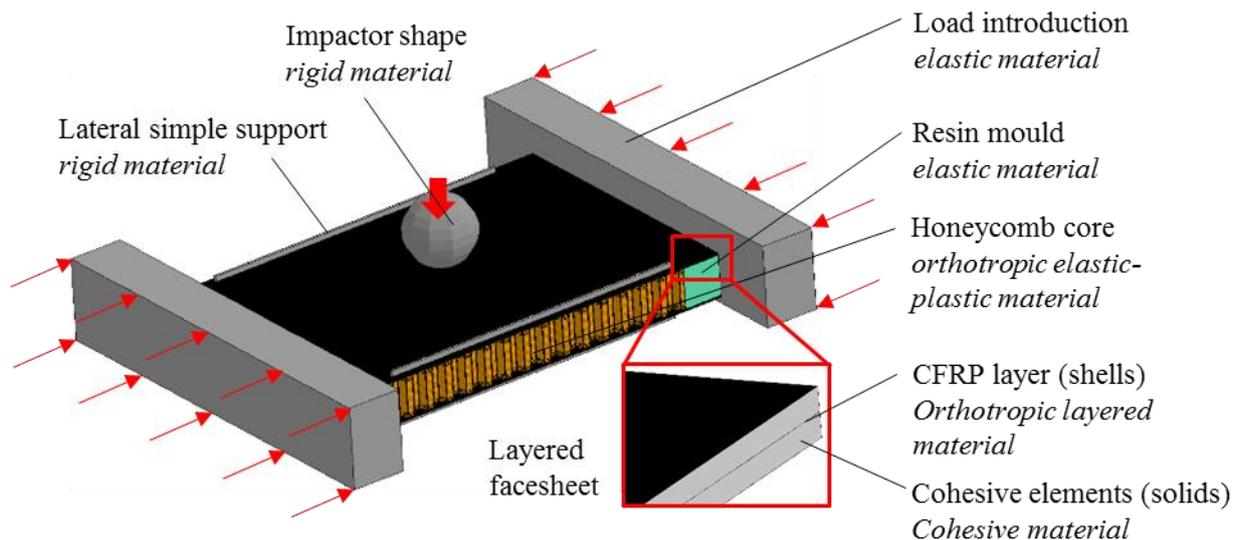
**Figure 5.** Finite element model for impact simulation
