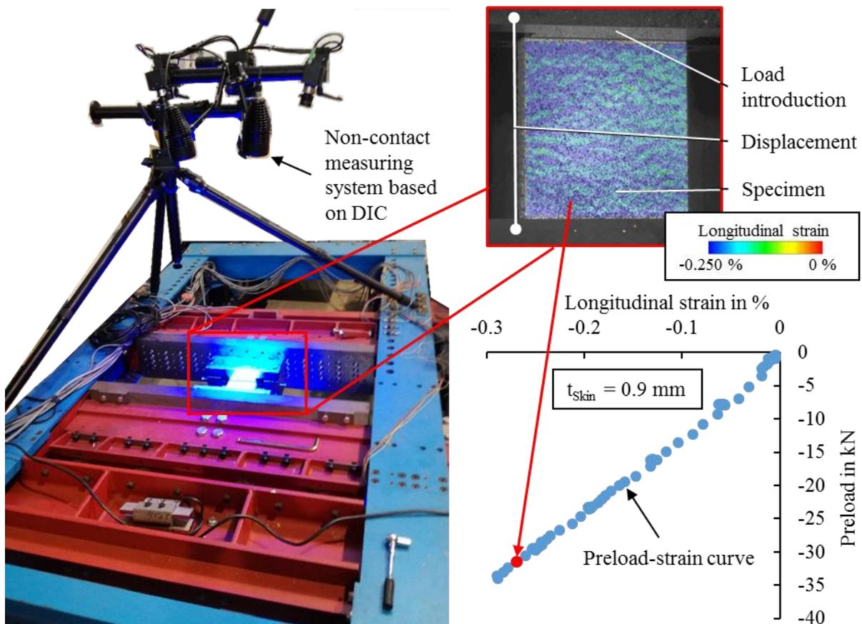
**Figure 2.** Test set-up for measuring the preload-strain behaviour
