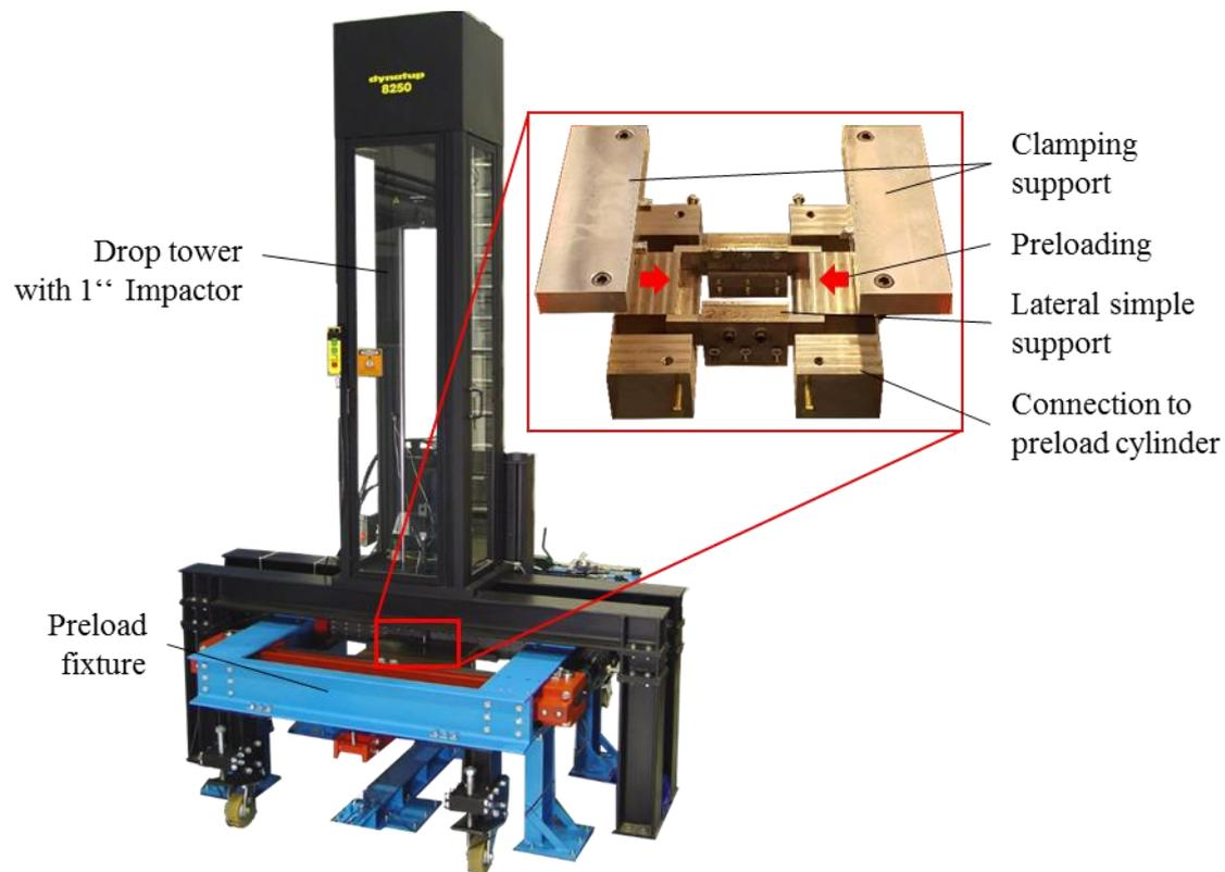
**Figure 3.** Preload and impact test set-up
