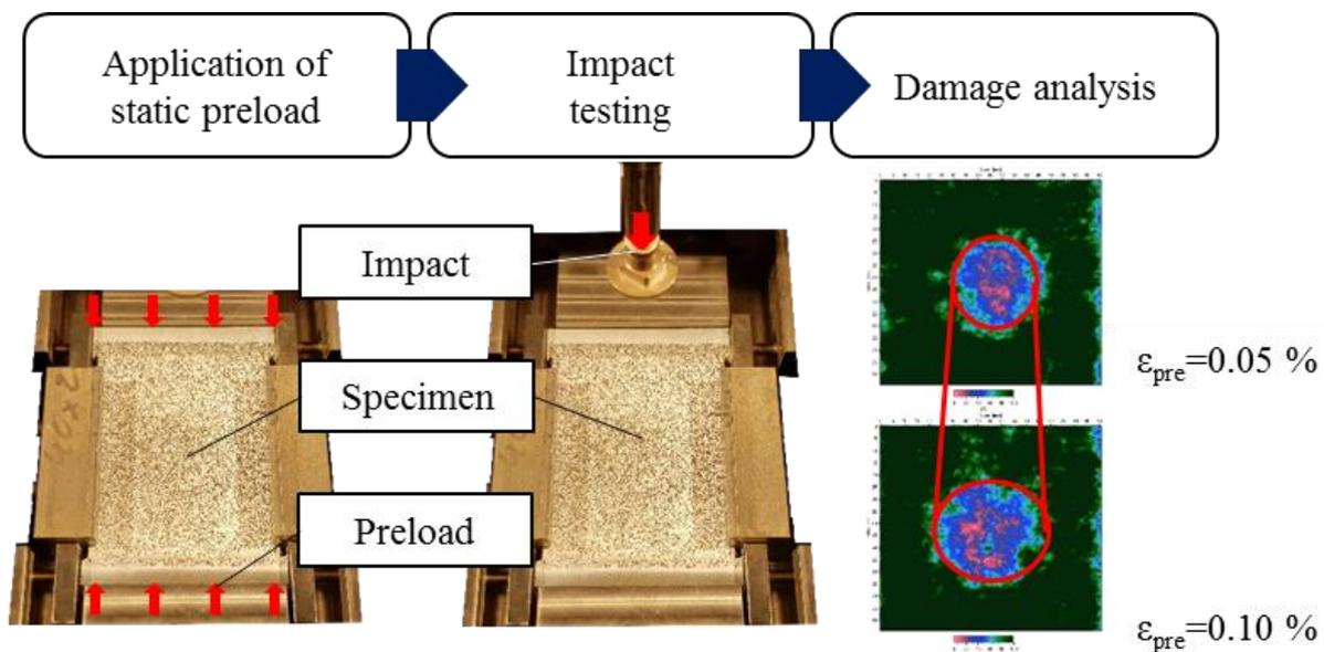
**Figure 1.** Procedure for impact tests on prestressed honeycomb sandwich structures
