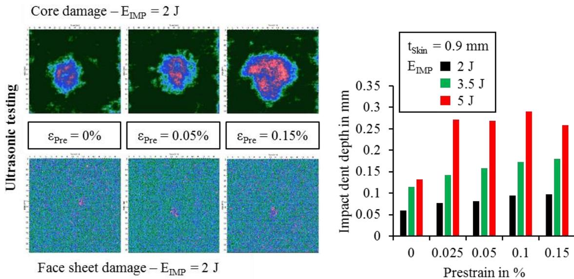
**Figure 4.** Ultrasonic damage images and dent depths of preloaded honeycomb sandwich structures
