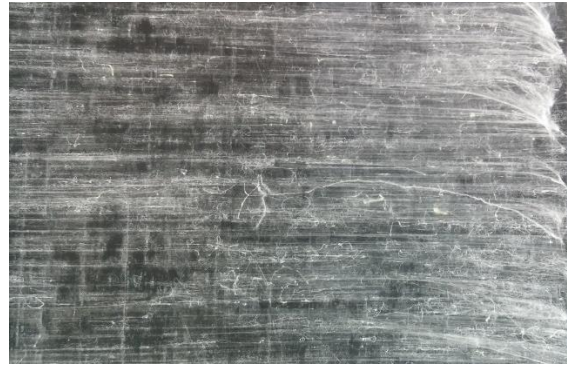
Figure 1: FibroTend, nylon 6,6 TNFs directly electrospun deposited on the CFRP composite surface
