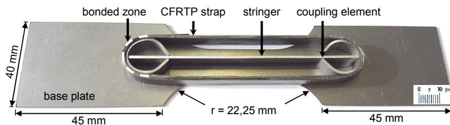
**Figure 2.** Geometry of the test specimen
