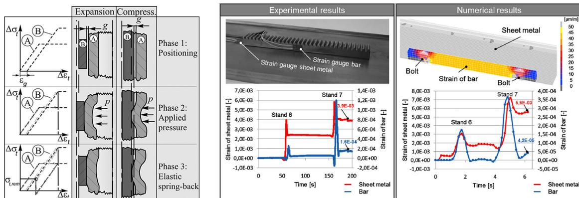
**Figure 1.** Force-closed joining by expansion and compression (left) [7] and by linear flow splitting (right) [8]
