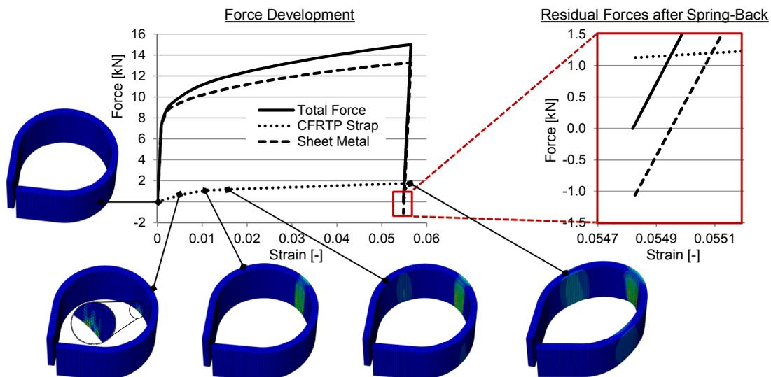
Figure 6. Development of the forces transmitted by FRP and stringer sheet during elongation (top) and the according plastically strained areas of the coupling element (bottom)
