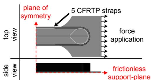
**Figure 4.** Numerical model of the tensile test
