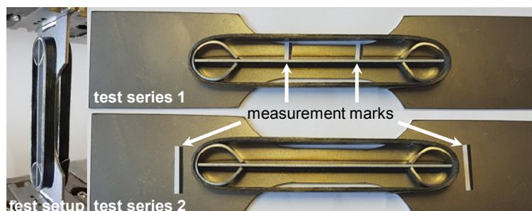
**Figure 3.** Test setup for the tensile tests (left) and measurement mark attachment points (right)
