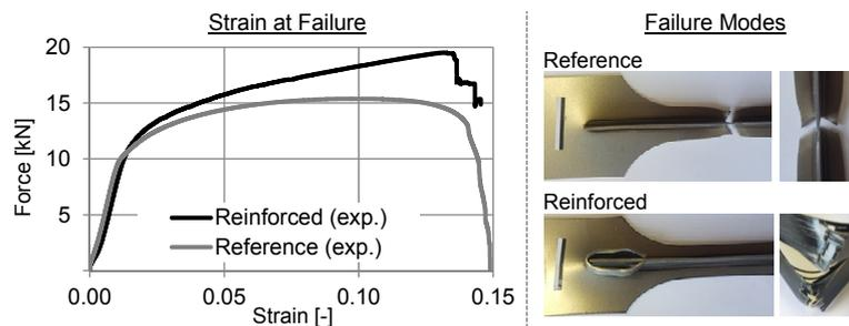
**Figure 7.** Comparison of the maximum endurable strain and failure modes
