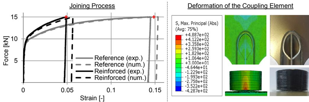
Figure 5. Comparison of the numerical and experimental results of the joining process
