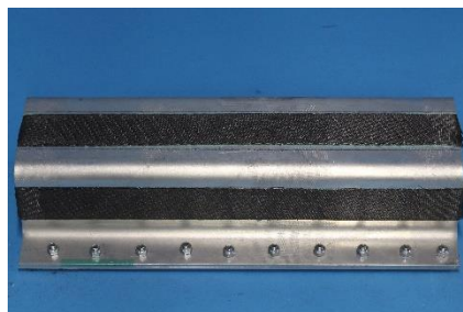
Figure 4. Crash tube with stripes.
