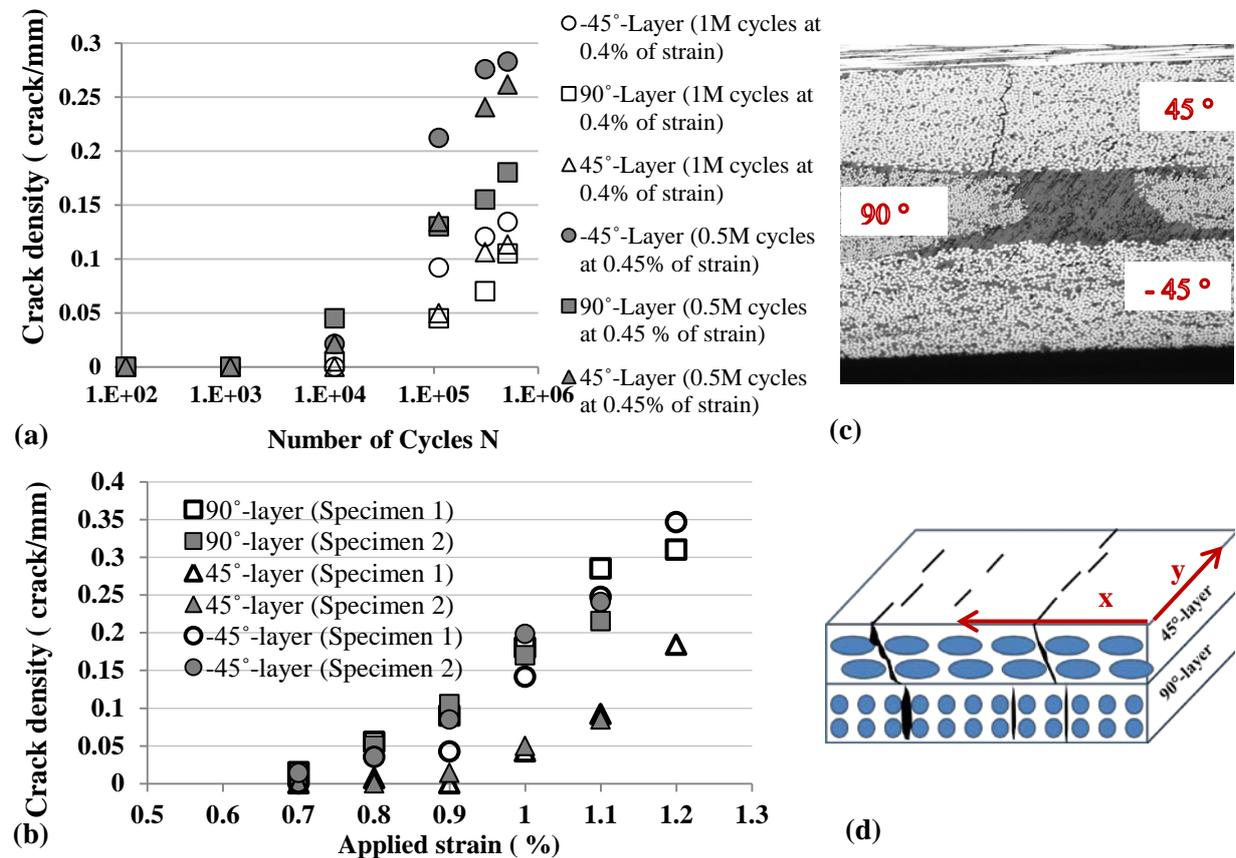
**Figure 3.** (a) Average transverse crack densities at the different layers of CF/EP [-45/90/45/0]s NCF at two different cyclic loading levels. (b) Average Transverse crack densities in the different layers of CF/EP [-45/90/45/0]s NCF subjected to quasi-static loading. (c) example of an edge 45°-layer crack where no other damage mode is observed. (d) Schematic view of 45°-layer crack.
