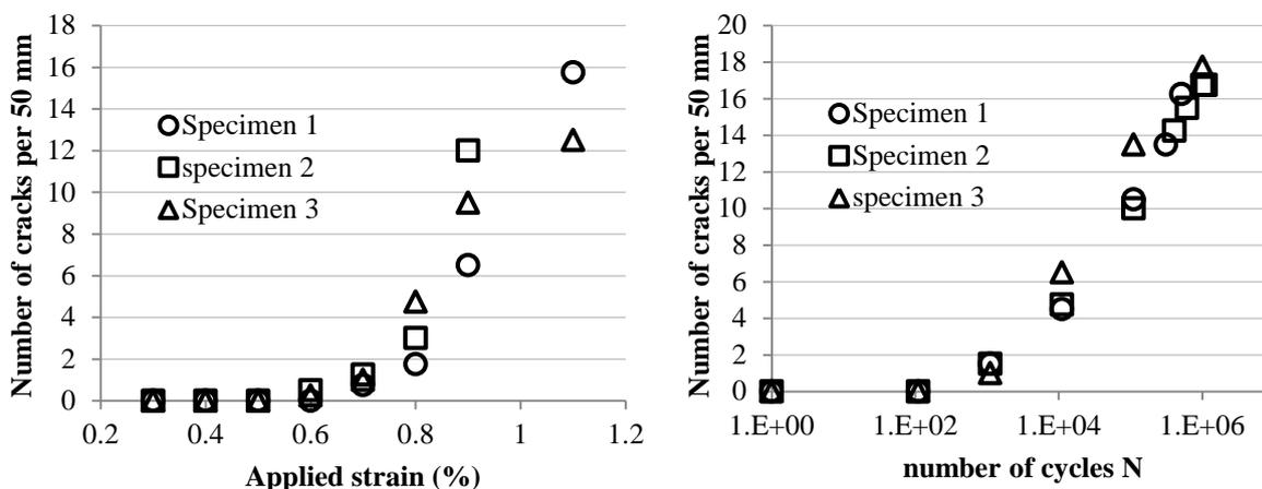
**Figure 2.** Dependence of the number of 90°-layer cracks over 50 mm length on the applied strain in quasi-static and on the number of cycles in fatigue loadings at 0.5% of max strain respectively.
