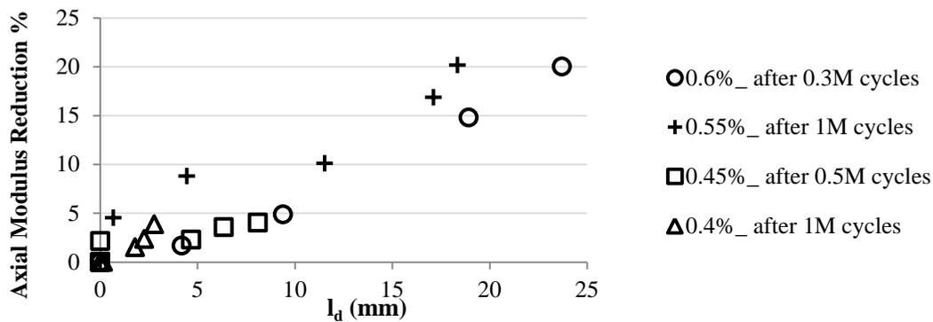
**Figure 6.** Axial modulus reduction dependence on average delamination length of the interfaces ±45/90 observed over a 50 mm of length.
