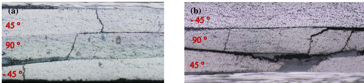
**Figure 4.** (a) Delamination migration at the interfaces after 1% strain of quasi-static loading. (b) Delamination at both interfaces after 0.5 M cycles at 0.55% of max strain at fatigue.
