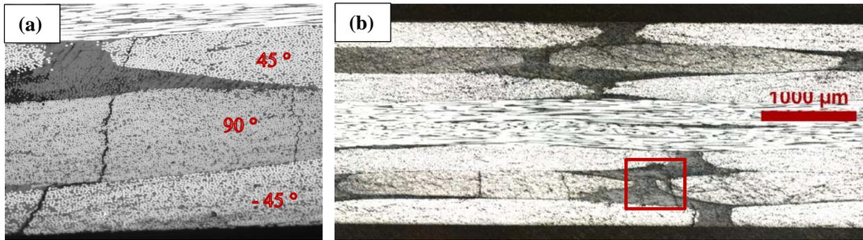
**Figure 1.** (a) Example of damage state after 1M cycles at 0.4% of maximum strain. (b) Stitch related crack in the 90°-layer.
