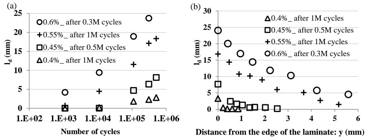
**Figure 5.** (a) Evolution of the average delamination length between the neighboring interfaces of the 90°-layer as a function of fatigue cycles. (b) Dependence of the average delamination length of both 90°/±45° interfaces on the number of cycles at different maximum strain level in fatigue.
