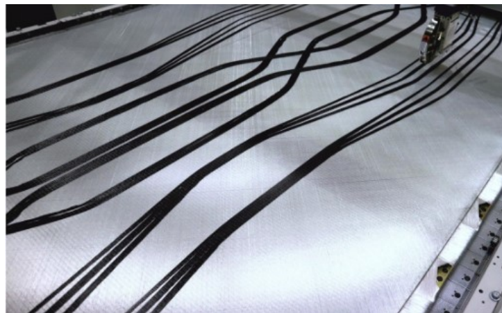
Figure 1. The load-path adapted fabrics can be fabricated at an arbitrary geometrical complexity
