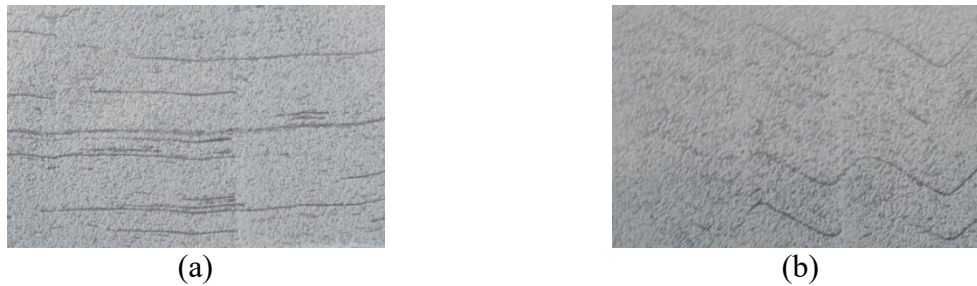
Figure 5. Applied powder with a coating thickness of 100 \mu\text{m} : Fixed doctor blade (a) and oscillating relative movement of the doctor blade (b)
